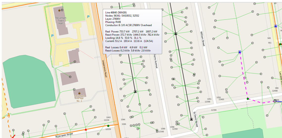
Figure 5. SmartMap's Load Flow Analysis calculates system loading, which is used to determine remaining capacity on a feeder.
