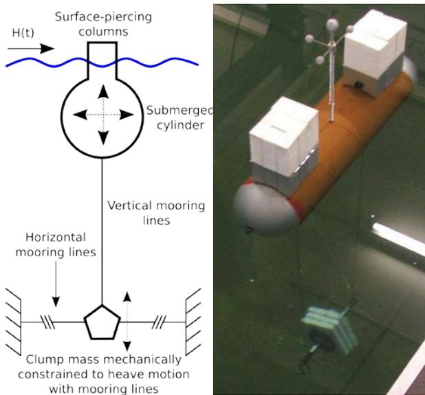
**Figure 1. (Left) Schematic of the experimental setup. (Right) Illustration of the experimental device (adapted from [1]).**
