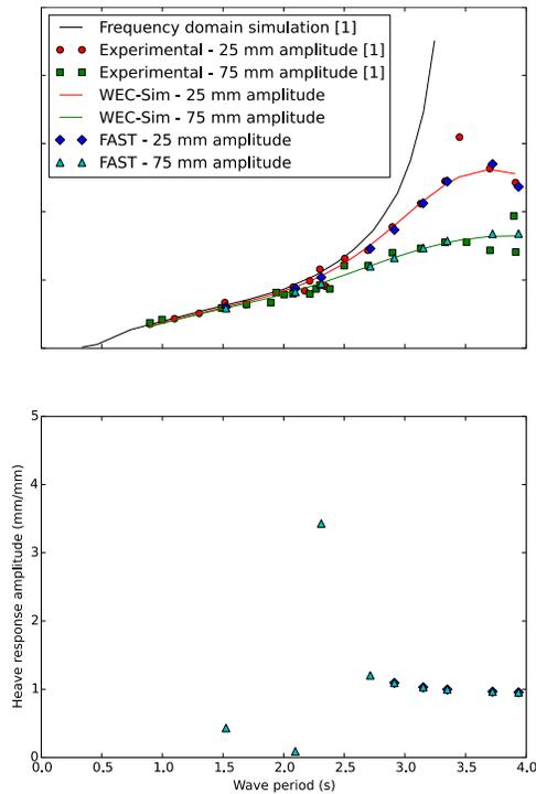
**Figure 8.** Response amplitude operator plots for surge (top) and heave (bottom). The plots show a comparison of the results from the frequency-domain simulations with no viscous drag [1], experimental data [1], WEC-Sim simulation results, and FAST simulation results.
