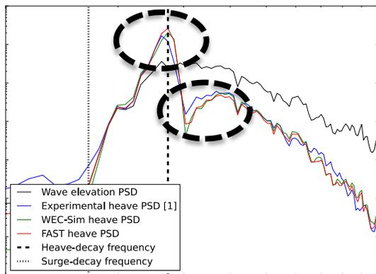
**Figure 12.** PSD of the heave motion calculated using results between 250 and 500 s. Note that the wave PSD and device natural frequencies are also shown for reference. The dashed lines identify regions where there is significant disagreement in the heave response PSD plots.
