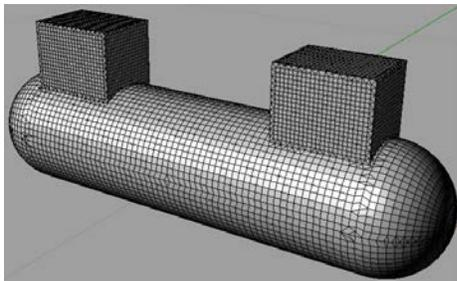
Figure 3. Panel mesh used for WAMIT simulations.
