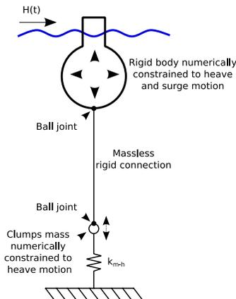
Figure 5. Schematic of the WEC-Sim model setup.
