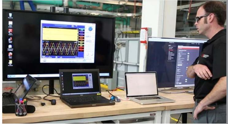
The ESIF's unique power hardware-in-the-loop capability allows Advanced Energy to evaluate its inverter's advanced grid support features and their impact on an electric distribution system prior to field deployment. *Still from DOE video*
