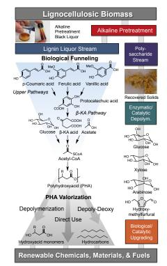
Illustration of how alkaline pretreatment was used to produce a lignin-enriched stream, which was then subjected to biological funneling to produce mcI-PHAs, which can serve directly as a bioplastic, be depolymerized to chemicals, or catalytically converted to fuels. Image by Derek R. Vardon, NREL
