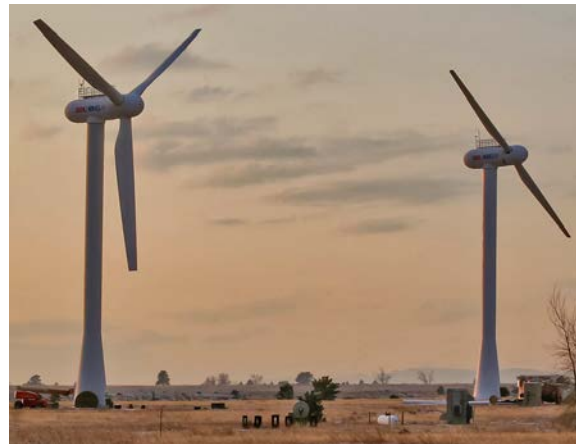
NREL's three-bladed Controls Advanced Research Turbine (CART3) and the two-bladed CART2, are used to test new control schemes and equipment for reducing loads on wind turbine components. Photo by Lee Jay Fingersh, NREL 19937
