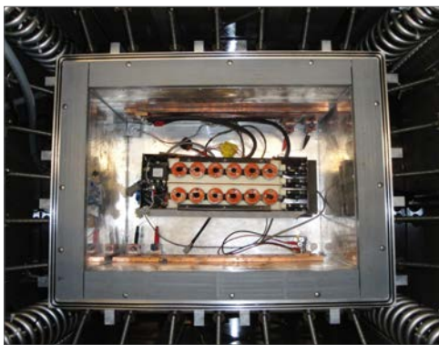
Left: A large battery module in the Large-Volume IBC test chamber, with cooling/heating coils in each corner. Photo by Dirk Long, NREL 6310097
