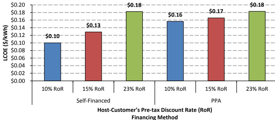
**Figure 9. Modeled LCOE of commercial PV systems: self-financed versus PPA, with varying discount rates**
