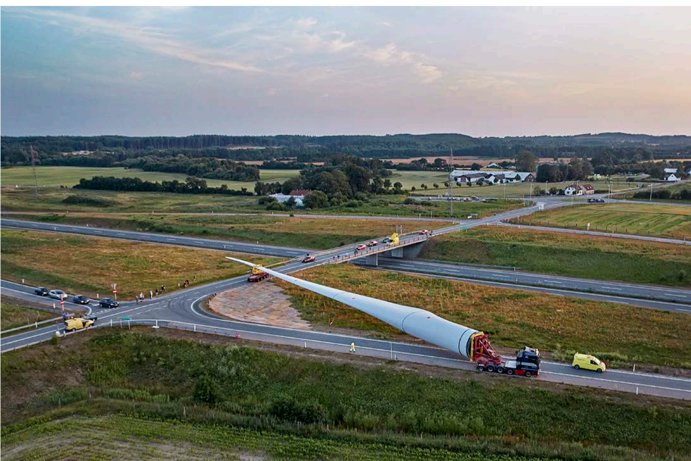
Figure 2-38. Example of wind turbine blades transportation obstacles
