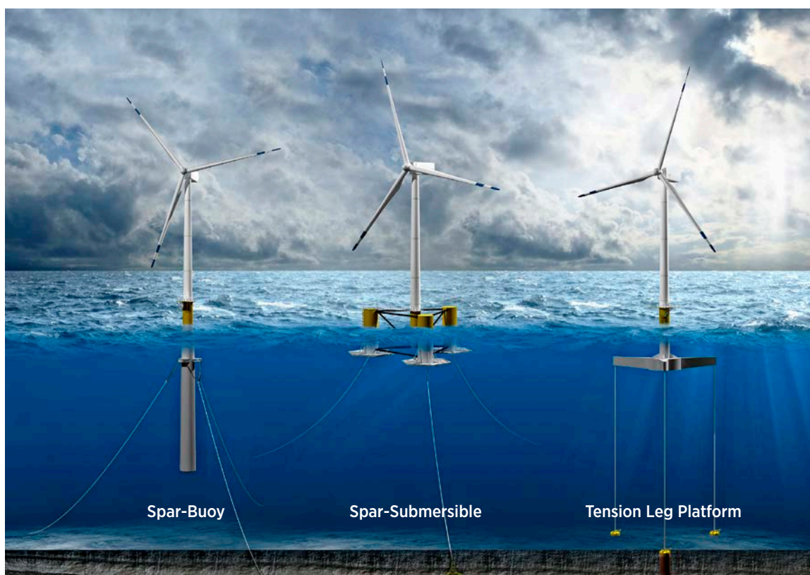
Figure 2-34. Illustrations of three classes of floating wind turbine technology
