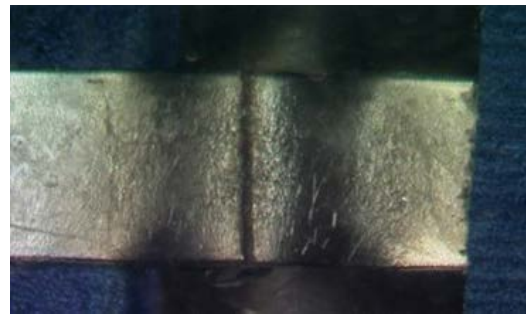
Figure 2: Picture of broken interconnect ribbon in module
