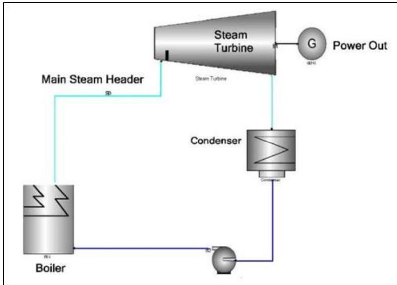
**Figure 3. Power generation-only biomass energy system (Note that the cooling tower is not shown.)**
