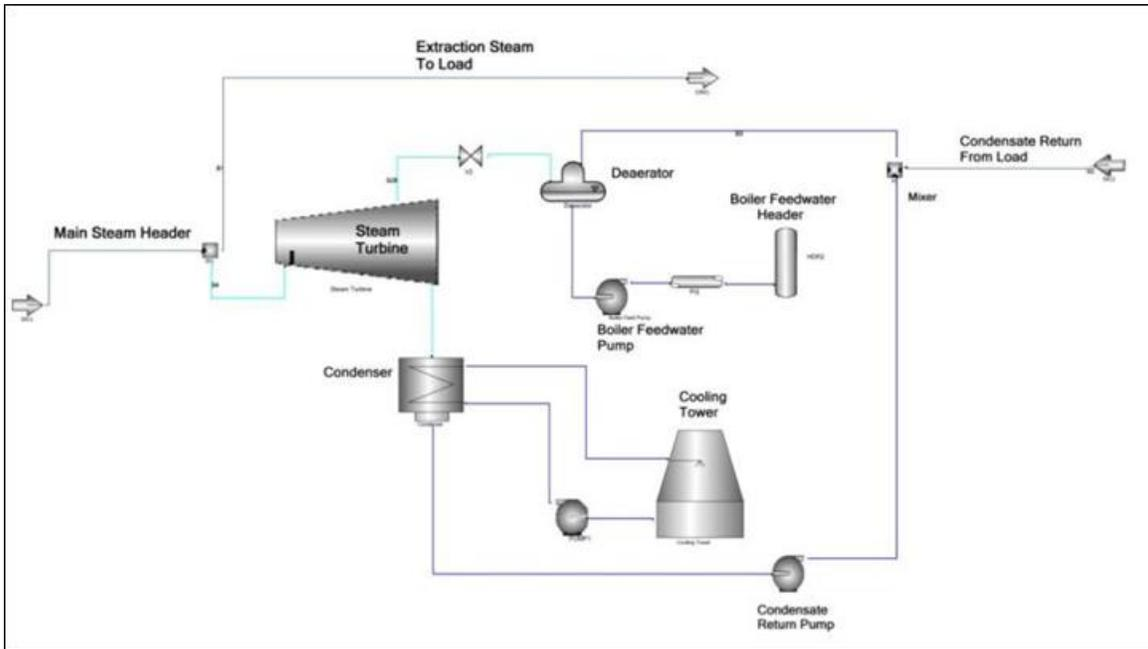
**Figure 4. CHP main steam extraction**
