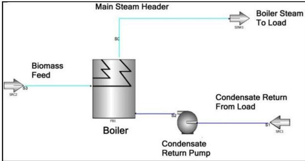
Figure 2. Thermal-only biomass energy system
