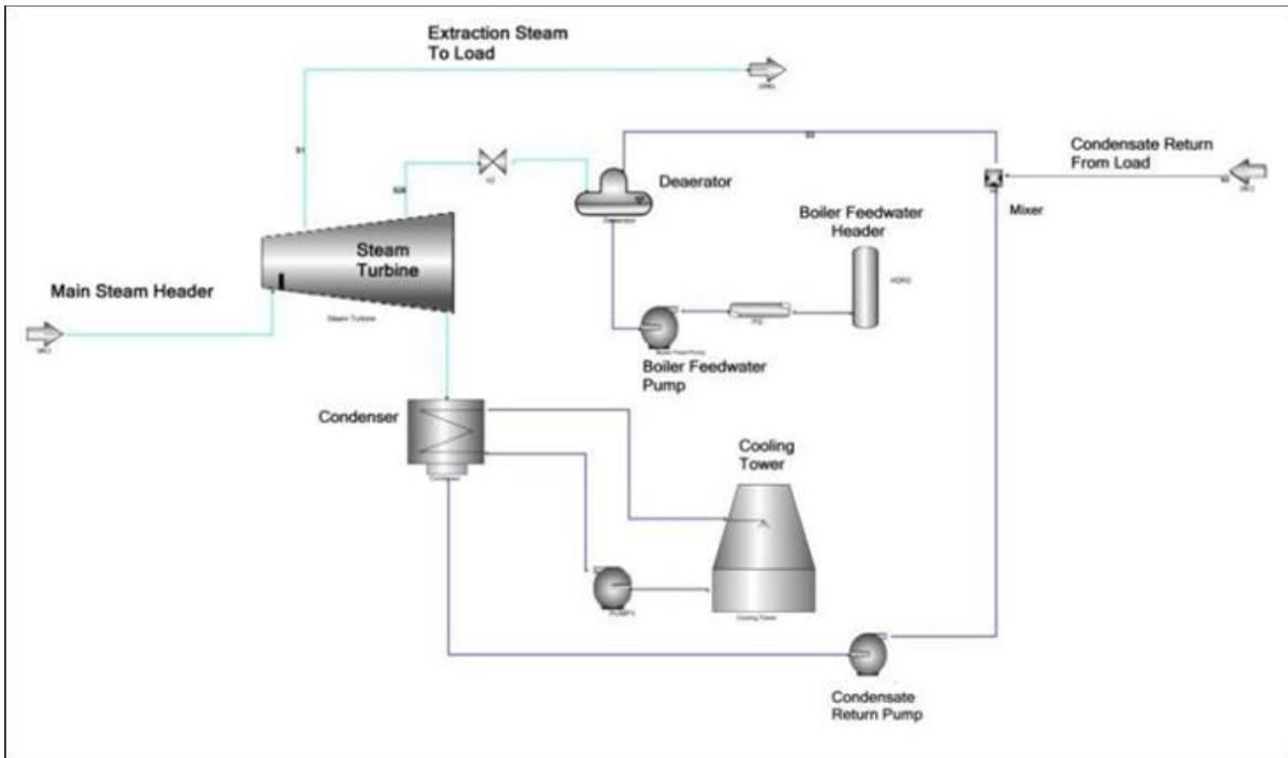
**Figure 5. CHP extraction turbine**
