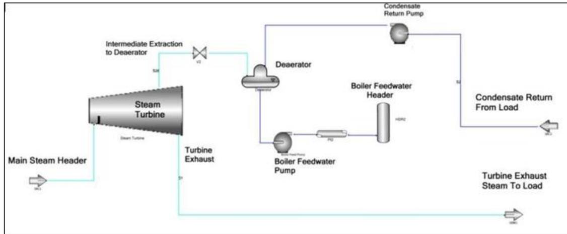
Figure 6. CHP backpressure turbine
