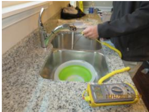
Figure 32. Tester measuring tap water temperature before test
