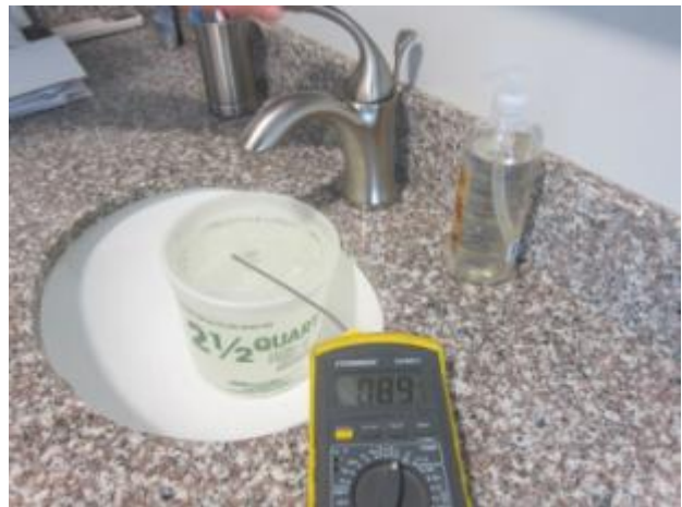
Figure 34. DHW wait time testing (end)
