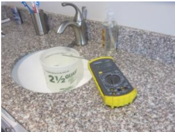
Figure 33. DHW wait time testing (start)
