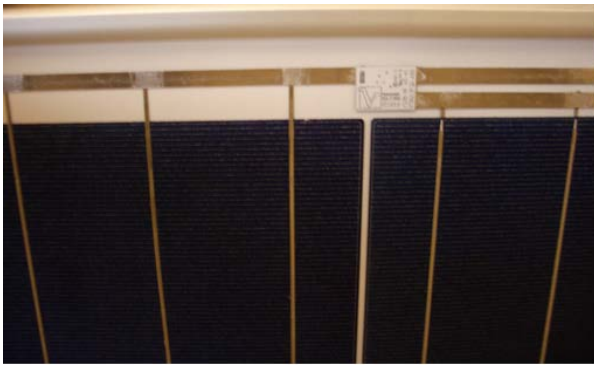
Fig. 2: Maxim VT8012 chipset embedded in the PV laminate. This “smart module” includes submodule power conversion in place of backplane diodes. Six of these DC-DC converters are integrated into each VT8012 PV module.
