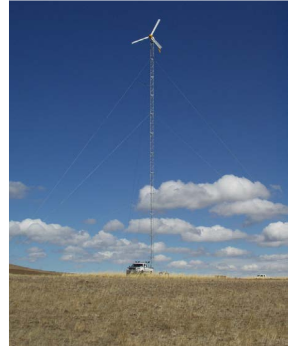
Bergey Excel 10, 10-kW turbine, Klickitat County, WA Photo by Gwen Bassetti, NREL 26429
