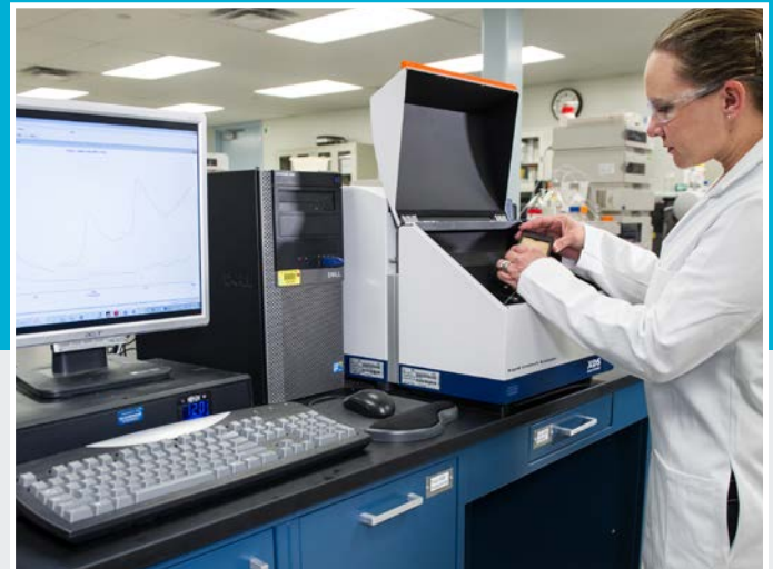
Scientists at NREL use near-infrared spectroscopy to predict the composition of a variety of biomass types.
