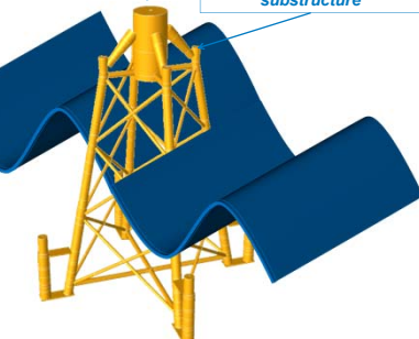
Figure 5. SACS adds substructure hydrodynamic loads and computes substructure overall overturning moment and stresses.
