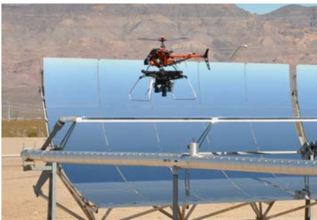
To find flaws in parabolic trough mirrors, a small-scale commercial helicopter with a specialized camera is part of the Distant Observer photogrammetric data acquisition system. Photo from Benjamin Ihas, NREL 23115
