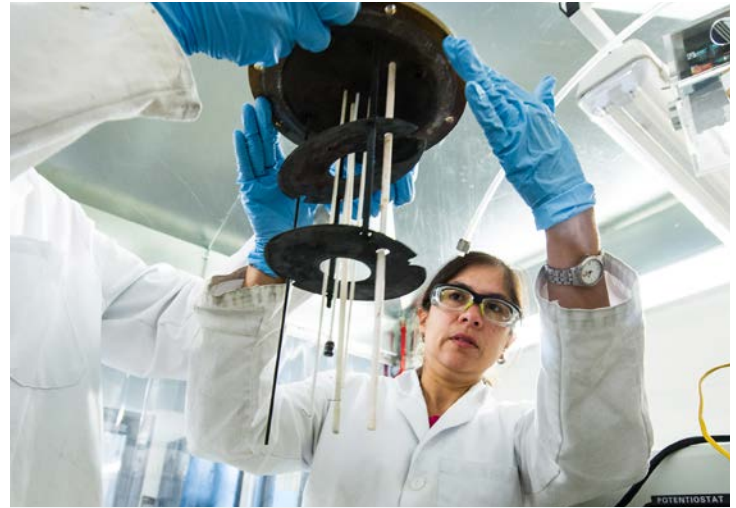
To advance thermal storage capabilities, NREL researchers use a three-electrode technique for evaluating high-temperature corrosion by molten salts. Photo by Dennis Schroeder, NREL 26587
