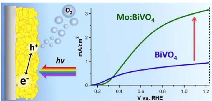
Doping nanoporous bismuth vanadate with molybdenum (Mo:BiVO<sub>4</sub>) improves the rate of majority carrier transport, dramatically increasing the water oxidation performance.
