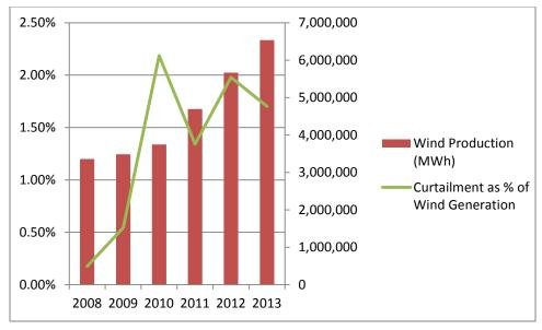
**Figure 5. PSCO wind curtailments as a fraction of total wind generation** Source: Xcel Energy (Bartlett 2013)
