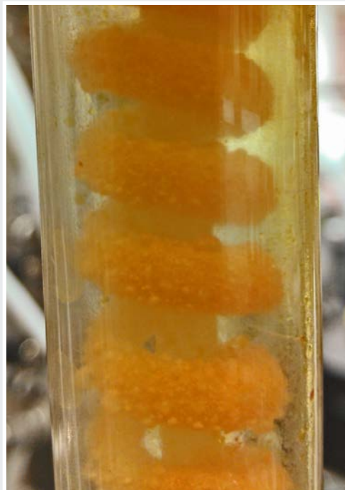
Glass condensers collect upgraded product vapors from the reactor for oil characterization.
