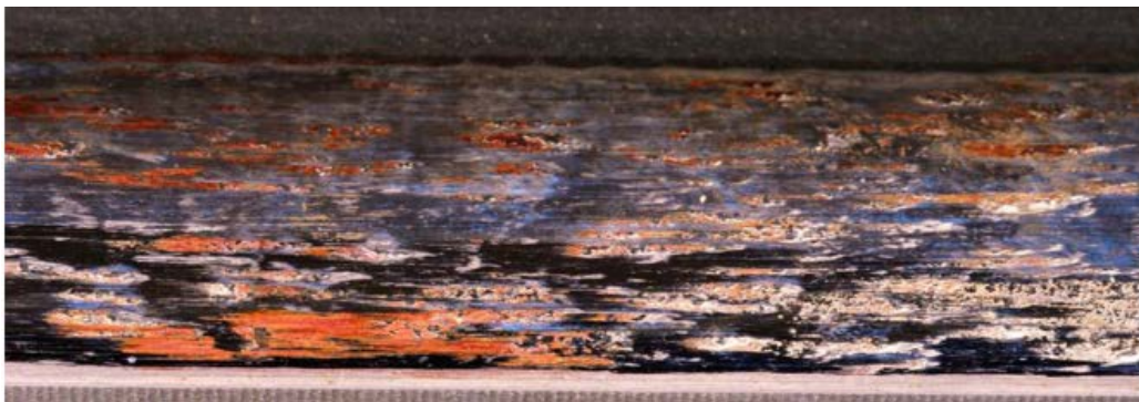
Figure 3. Close-up of fretting corrosion of the sun spline. Photo by Robert Errichello, GEARTECH, NREL 19853
