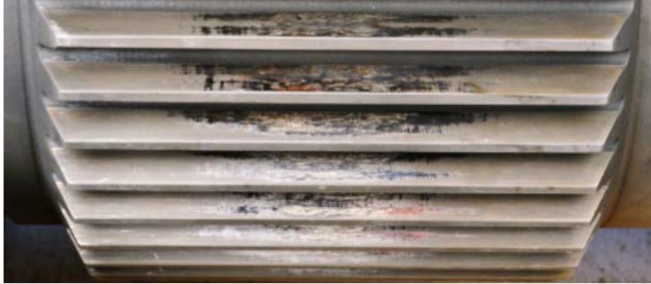
Figure 2. Fretting corrosion of the sun spline. Photo by Robert Errichello, GEARTECH, NREL 19852
