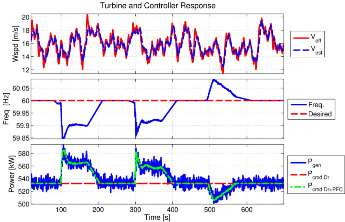
**Figure 4-8. Simulation results for a turbulent 16 m/s wind field with a de-rating command of 0.9 in de-rating mode 1, a droop curve slope of 2.5%, and deadband of 17 mHz. Recorded data from grid frequency events were passed into the controller near the 100-, 300-, and 500-second marks to show the PFC.**
