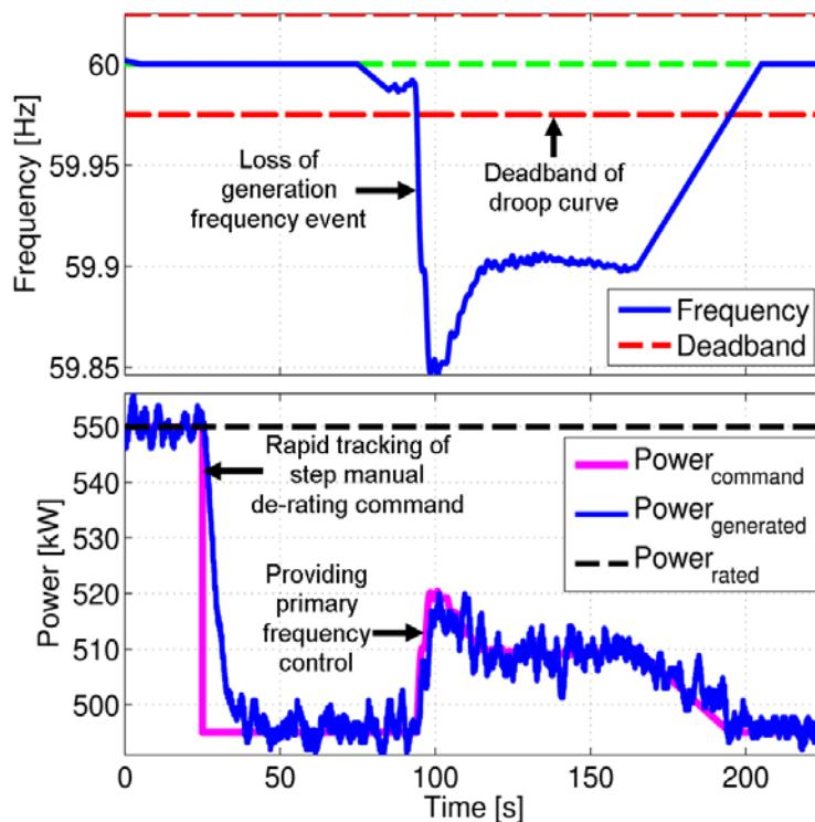
**Figure 4-15. Field test data that shows the turbine tracking a step change in the de-rating command followed by a PFC.**
