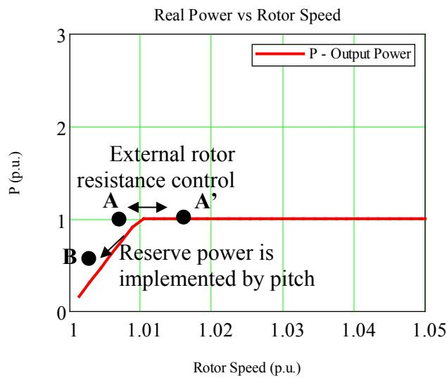
Figure 3-12. Output power versus rotor speed (Type 2 WTG).
