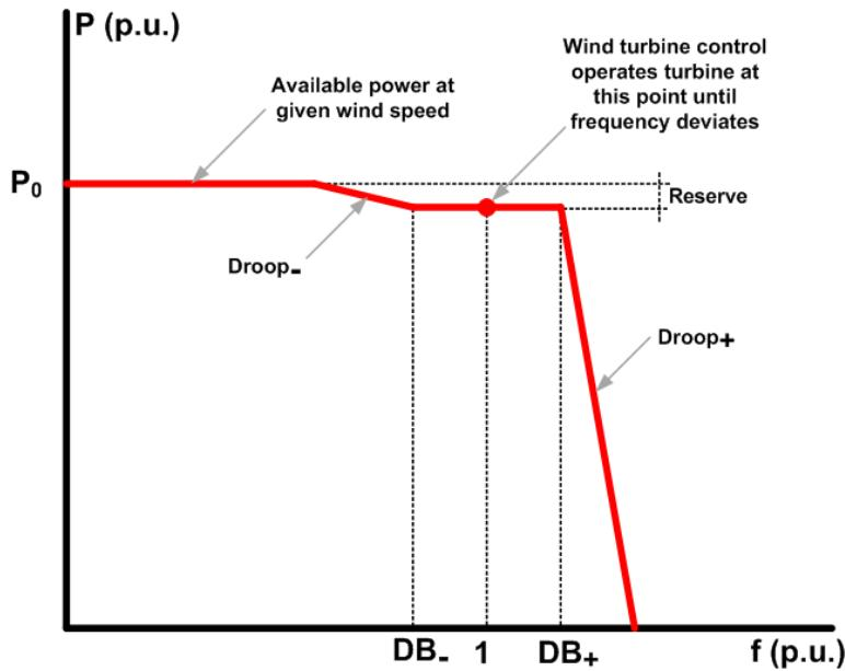
Figure 3-27. PFC implemented with a frequency droop on a wind power plant.
