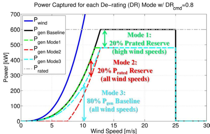
**Figure 4-3. A depiction of the steady-state power commands in each de-rating mode when a de-rating command of  $Dr_{cmd} = 0.8$  is used.**
