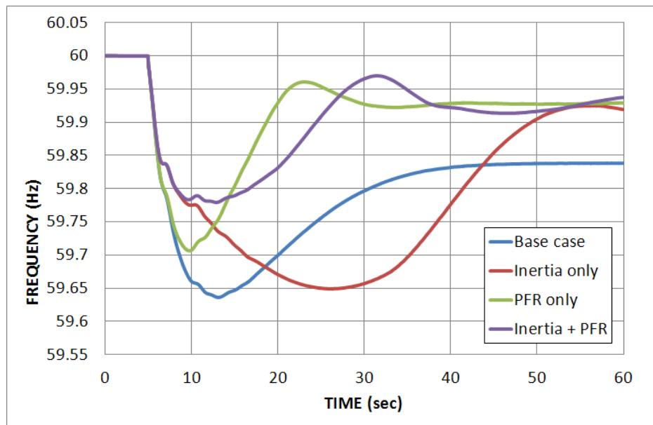
**Figure 3-44.** WI frequency response for 30% wind power penetration.
