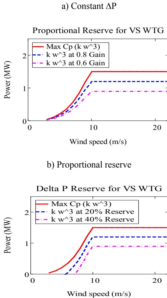
**Figure 3-22. The reserve power for a variable-speed WTG using two different methods.**
