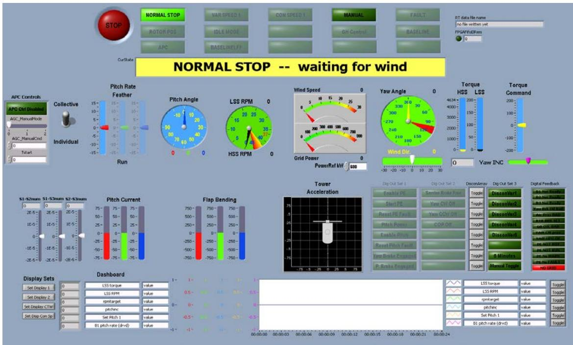
**Figure 4-13. The operator user interface for running the APC controller on the CART3 wind turbine. The APC-specific controls have been added to the left side of the user interface.**
