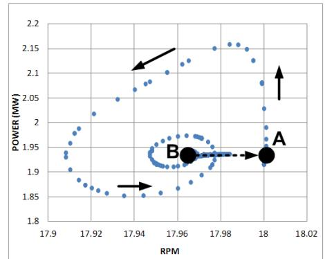
**Figure 3-9. Trajectory of operating point during a frequency decline for Type 1 WTG for a system with low inertia.**
