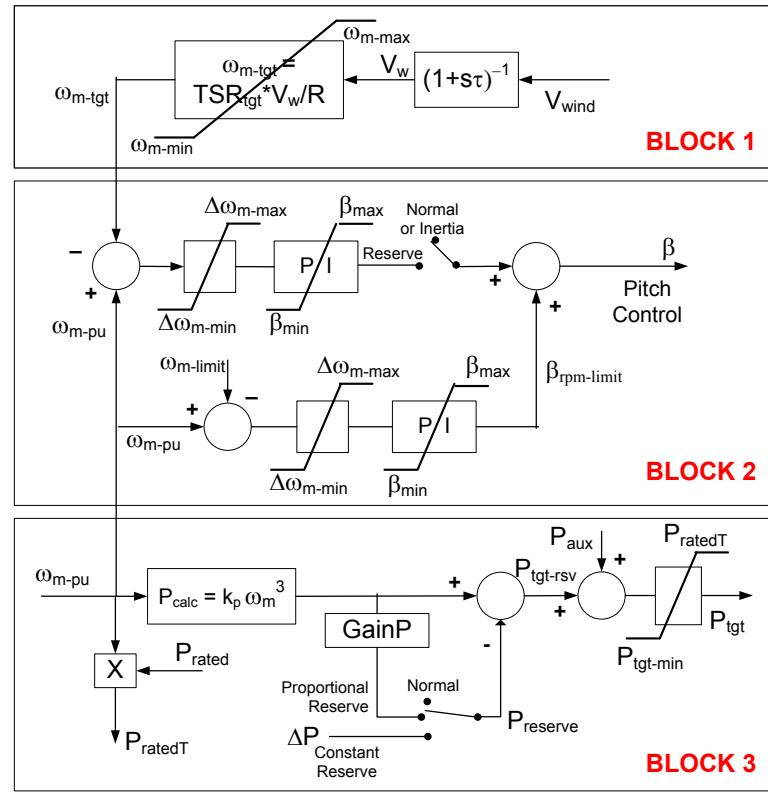
**Figure 3-24. Pitch controller and real power controller used to set reserve power for Type 3 and Type 4 WTGs.**
