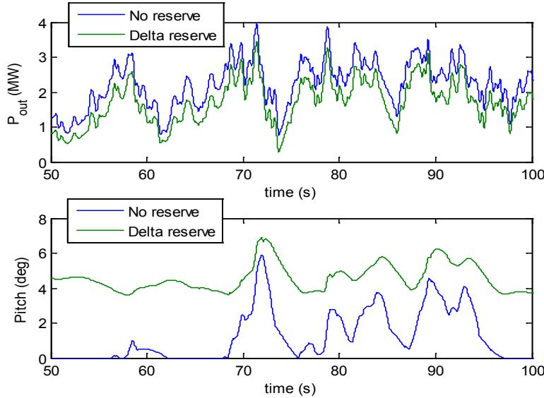
**Figure 3-15. Output power and pitch angle for constant reserve power ( $\Delta P_{\text{reserve}}$ ) implementation on a Type 1 wind turbine.**
