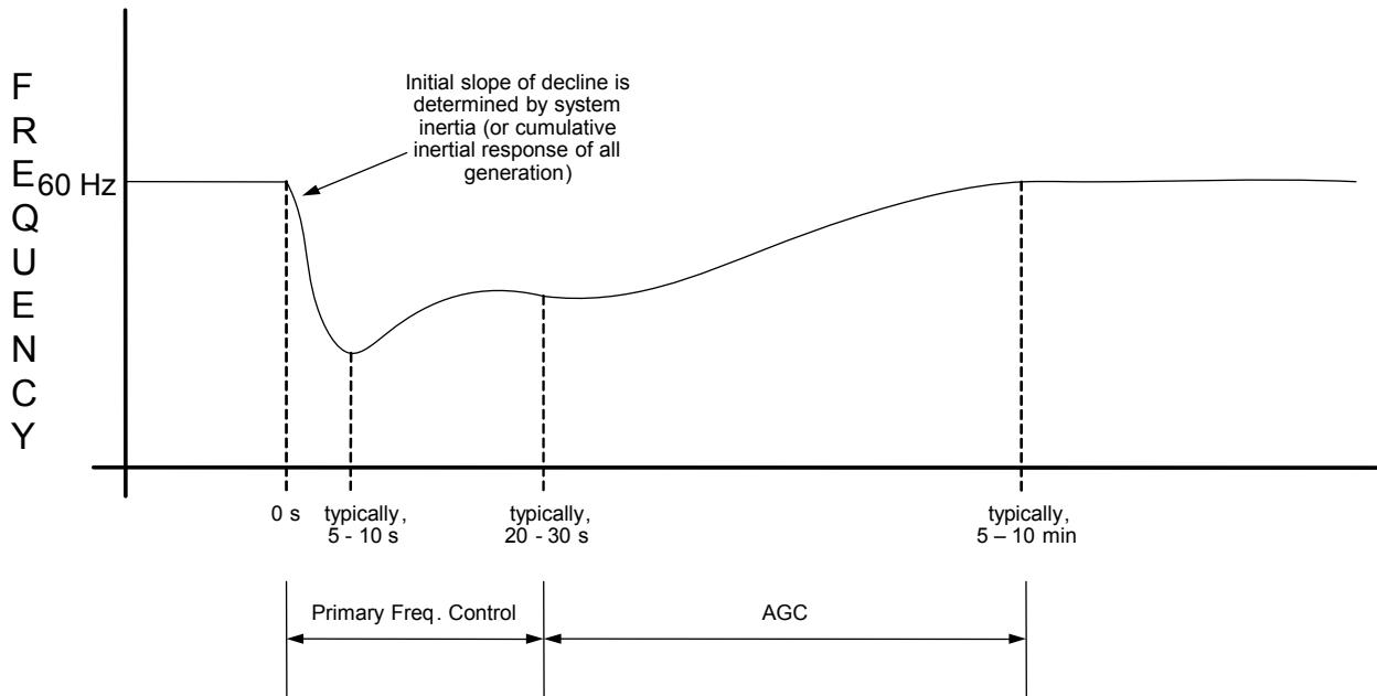
**Figure ES-2. Frequency trace following a large contingency event (i.e., loss of a large generating unit). Inertial control, PFC, and AGC (secondary frequency control) each serve a different purpose, and their response timeframes are also at different points of the frequency recovery.**
