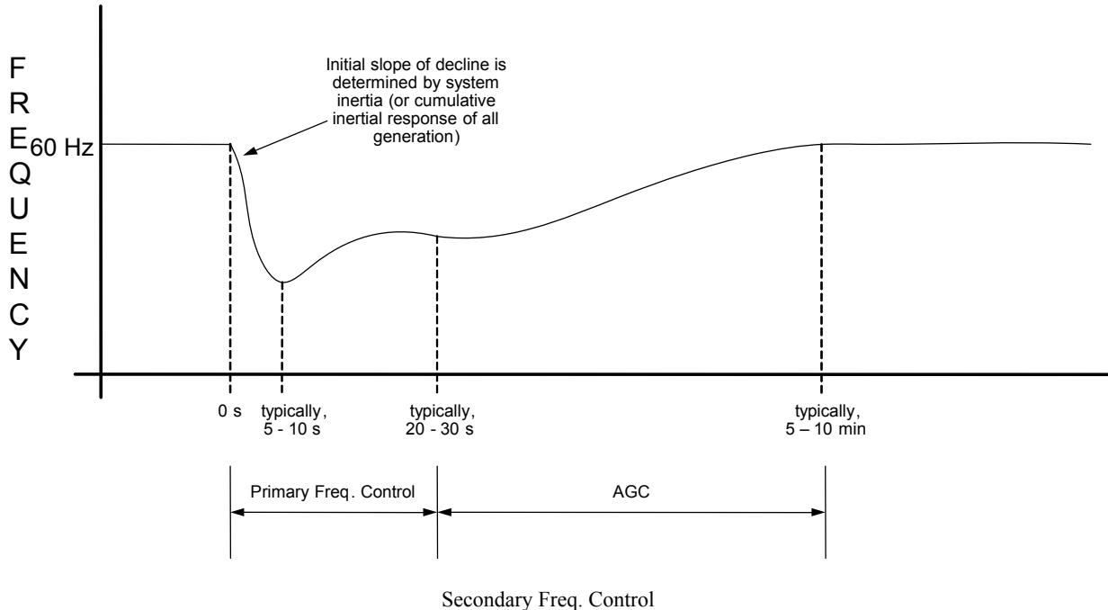
**Figure 1-2. Frequency trace following a large contingency event (i.e., loss of a large generating unit). Inertial control, PFC, and secondary frequency control each serve a different purpose, and their response timeframes are also at different points of the frequency recovery.**
