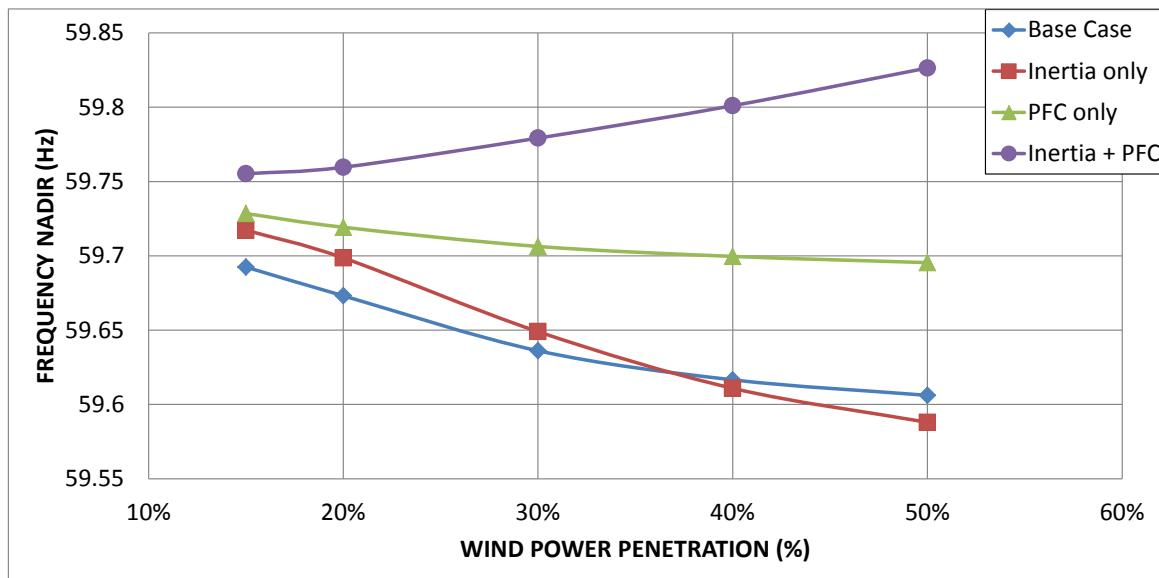
**Figure ES-5. Impact of wind power controls on frequency nadir.**
