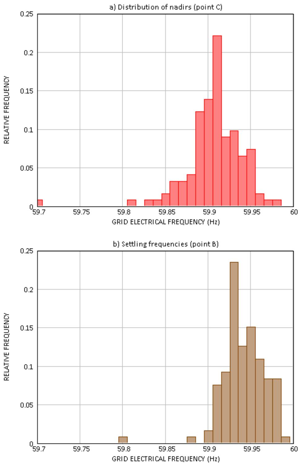
**Figure ES-4. Distribution of low-frequency event data. Point C is the frequency nadir and point B is the settling frequency.**
