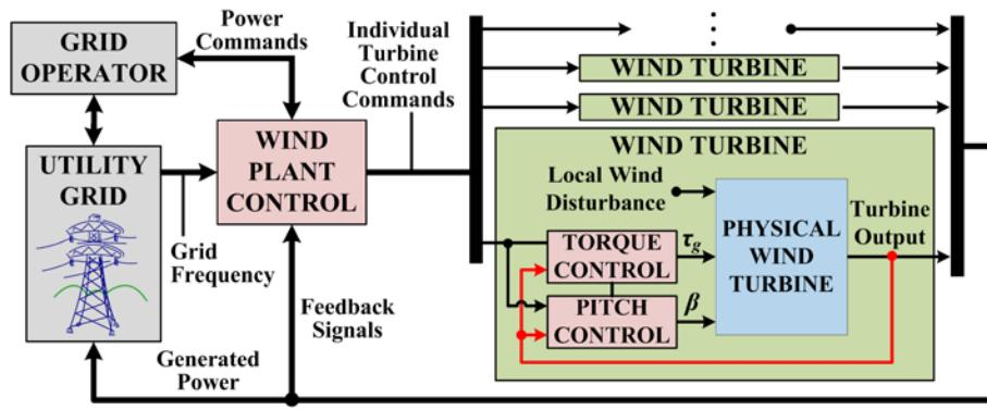
**Figure 4-1. A schematic that shows the communication and coupling between the wind plant control system, individual wind turbines, utility grid, and the grid operator.**
