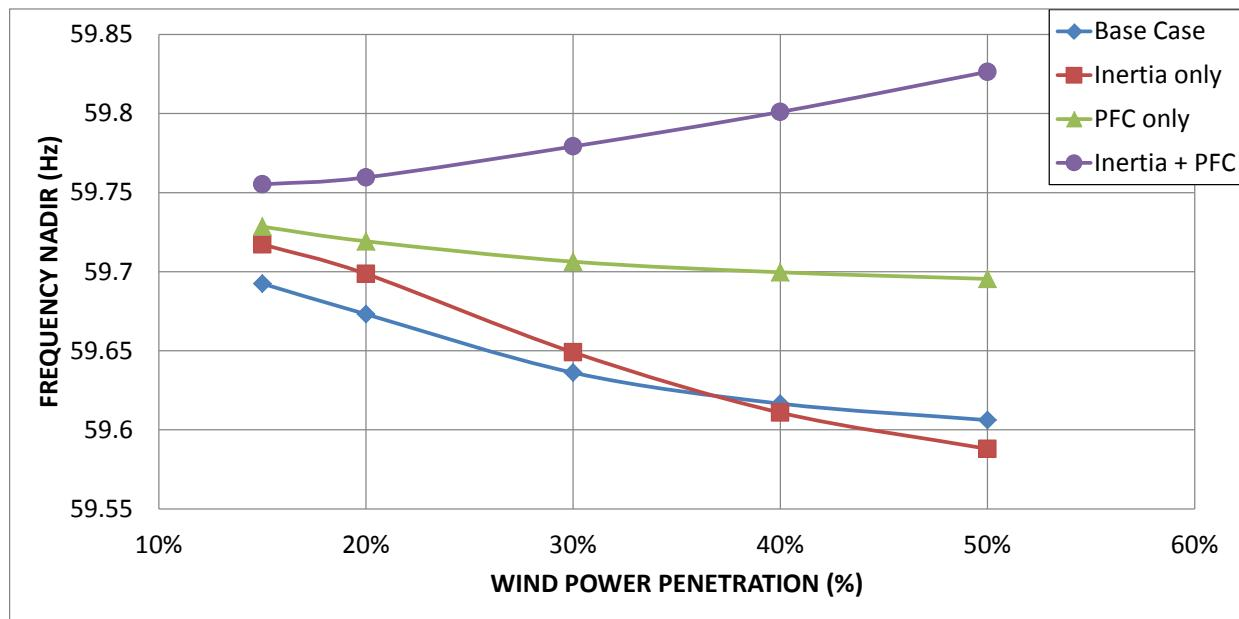
**Figure 3-47. Impact of wind power controls on frequency nadir.**
