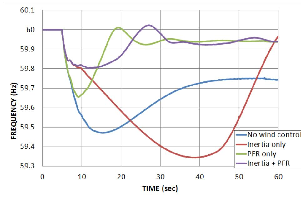
**Figure 3-55. Impact of wind power controls (50% penetration and  $K_t = 40\%$ ).**
