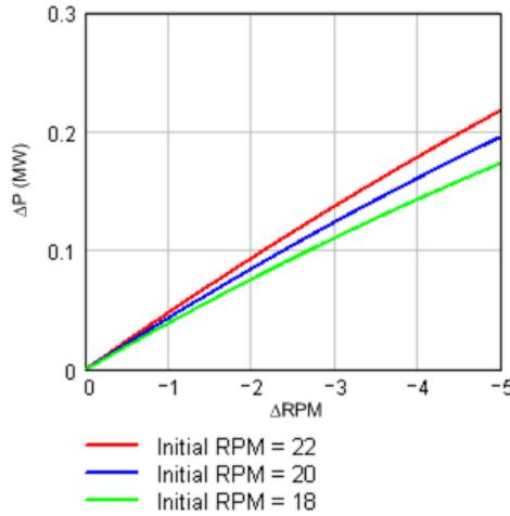
**Figure 3-2. Example dependence of  $\Delta P$  on RPM decline.**
