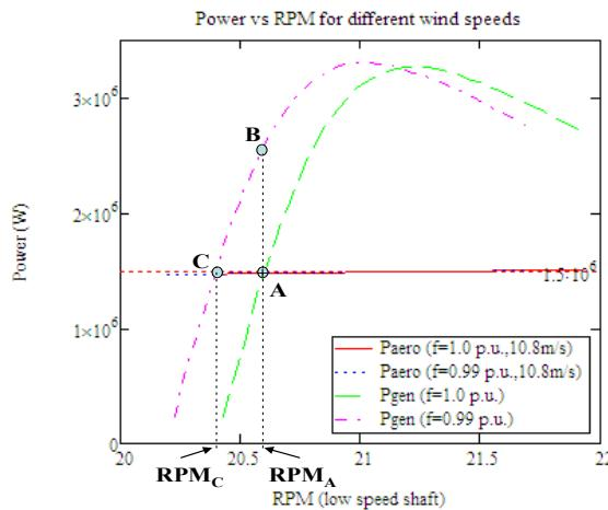
**Figure 3-3. Illustration of kinetic energy transfer during a frequency decline for Type 1 and 2 WTGs.**
