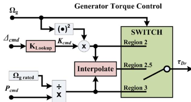
**Figure 4-6. A detailed schematic of the de-rating torque controller block.**
