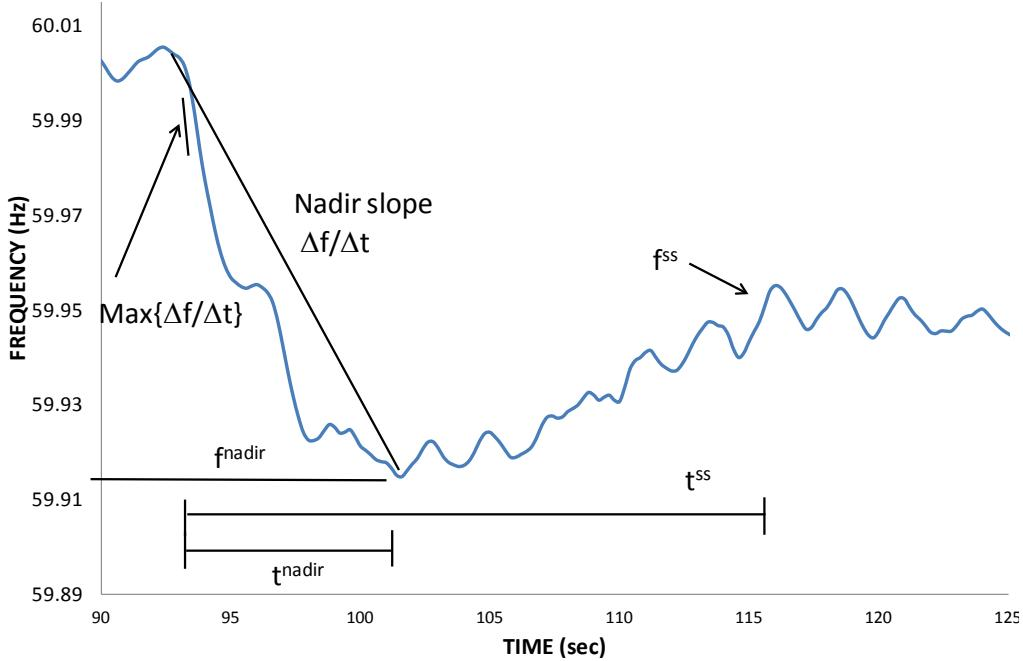
**Figure 2-1. Western Interconnection frequency during the first instances following a disturbance, and some metrics that can show the performance of PFC.**
