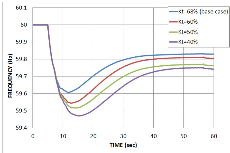
**Figure 3-54. Impact of  $K_t$  for 50% penetration case (wind providing no APC).**
