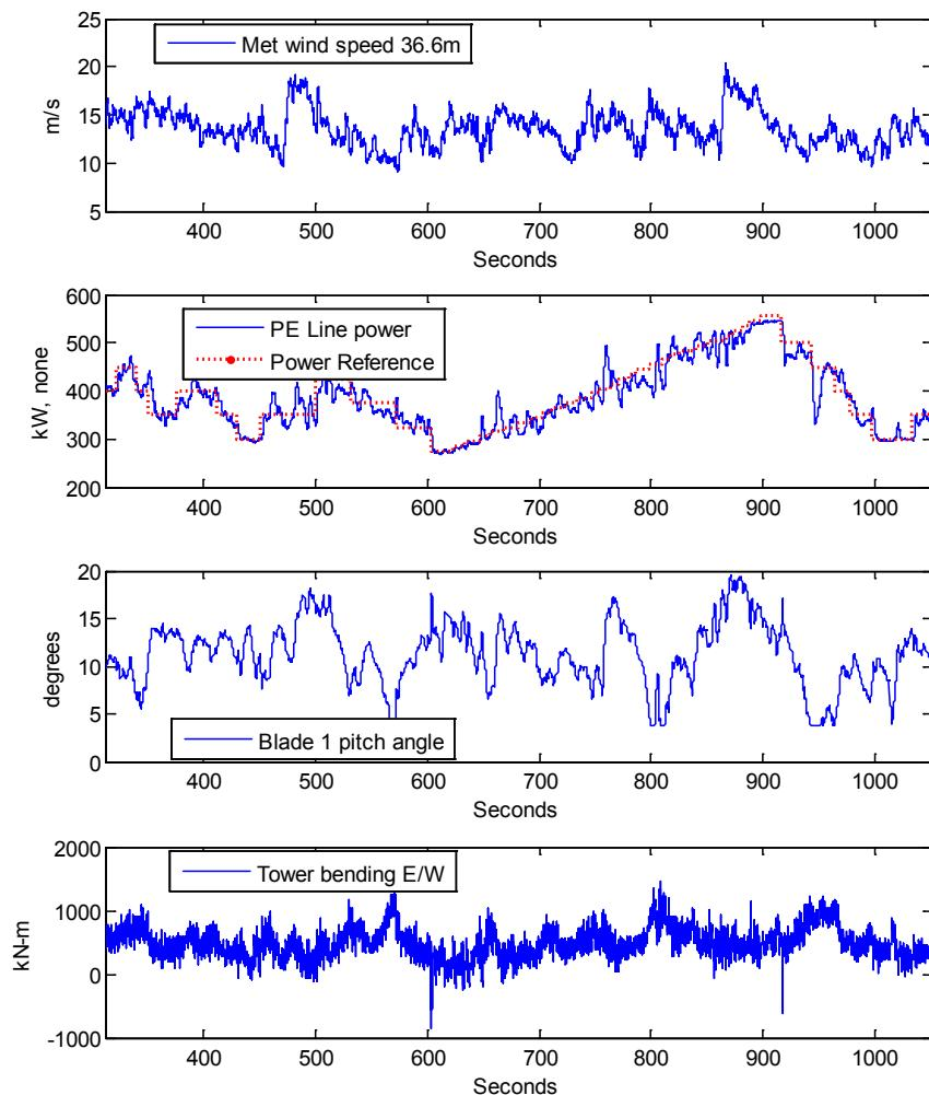
**Figure 4-11. Field test data of the FSC APC control system on CART3, showing reasonable trends in power reference following.**
