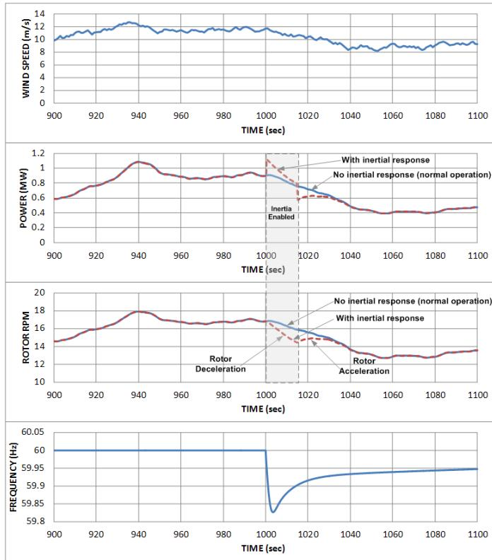
**Figure 3-20. Simulated example of Type 3 inertial response (lower power).**
