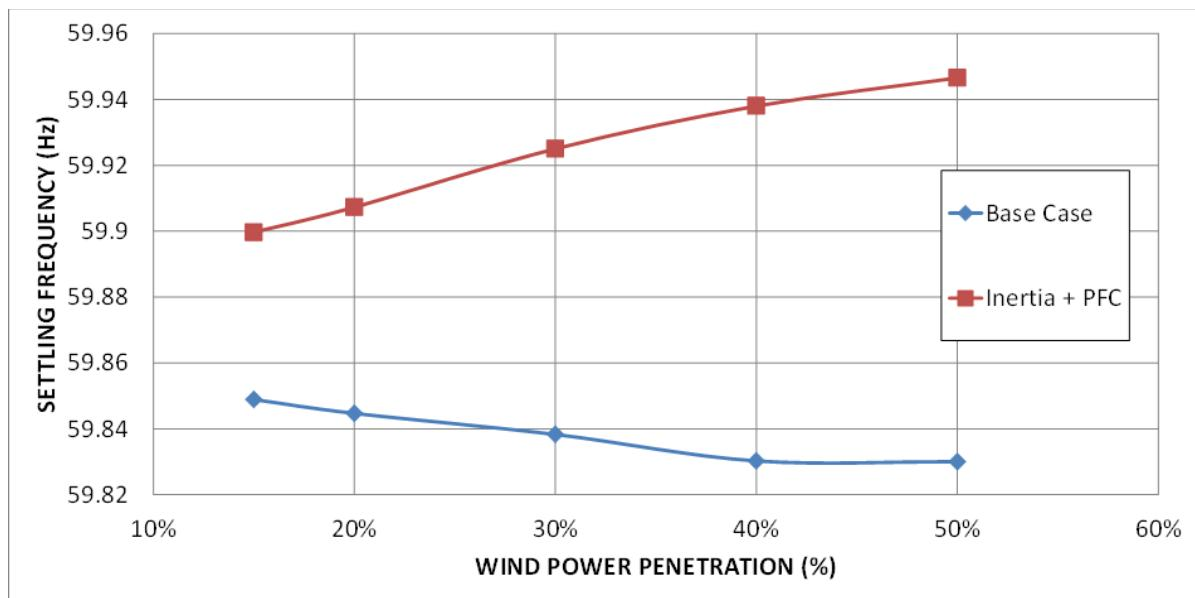
**Figure 3-48. Impact of wind power controls on settling frequency.**
