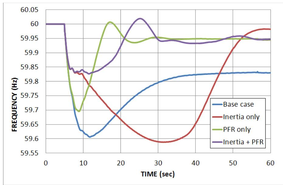
**Figure 3-46. WI frequency response for 50% wind power penetration.**
