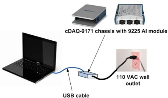
**Figure 3-28. NREL grid frequency monitoring system.**
