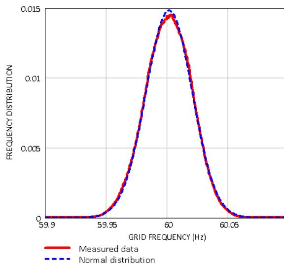
**Figure 3-38. Distribution fitting for continuous frequency data.**
