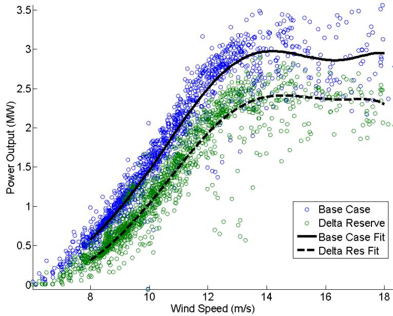
**Figure 3-17.** Output power comparison between the base case and delta reserve power of a Type 2 wind turbine based on the dynamic simulation with  $\Delta P_{\text{reserve}} = 20\%$  of the rated power.
