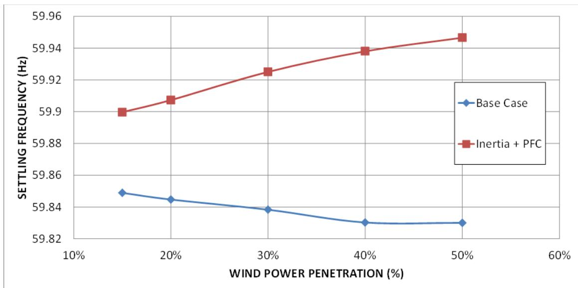
**Figure ES-6. Impact of wind power controls on settling frequency.**
