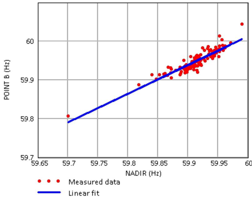
**Figure 3-37. Relationship between nadir (point C) and settling frequency (point B).**
