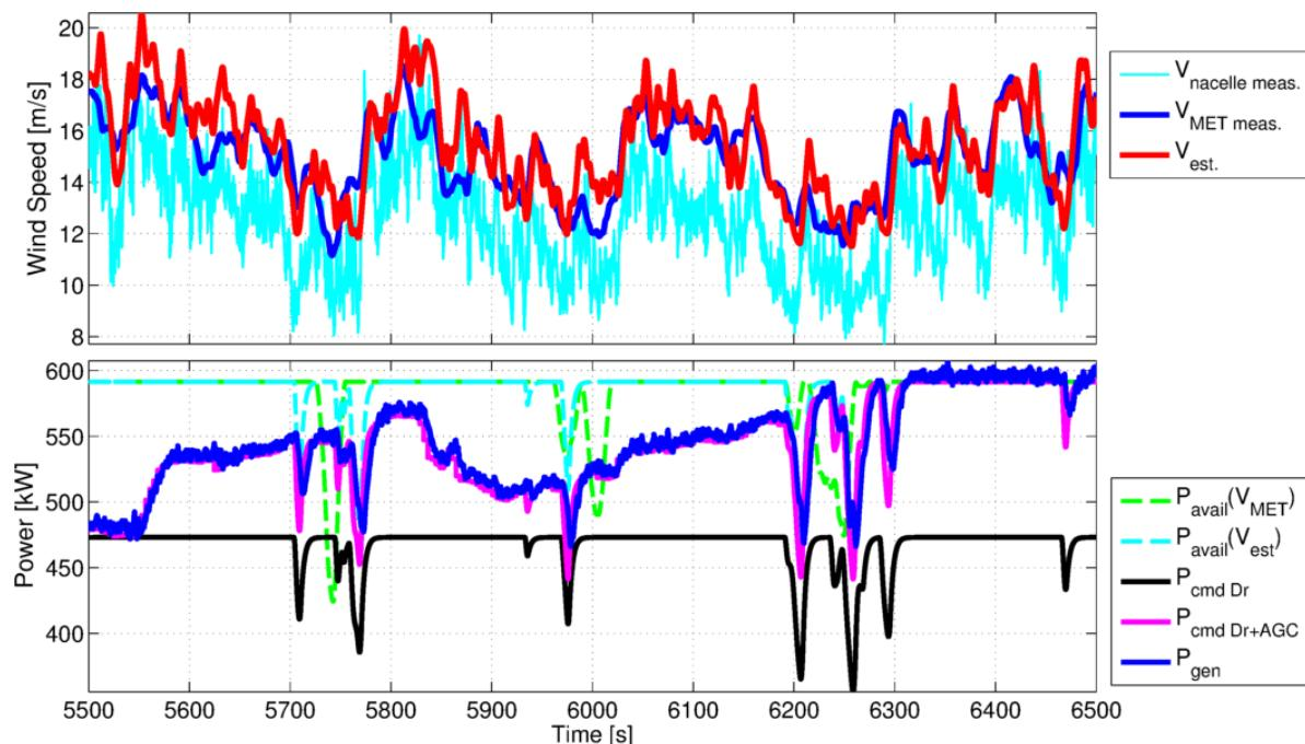
**Figure ES-9. A field test of the CART3 turbine following an AGC command.**
