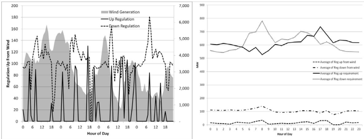
**Figure 2-8. Provision of regulation for four days in April (left), and averaged by hour for entire two-month study (right).**
