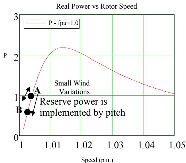
**Figure 3-11. Output power versus rotor speed (Type 1 WTG).**
