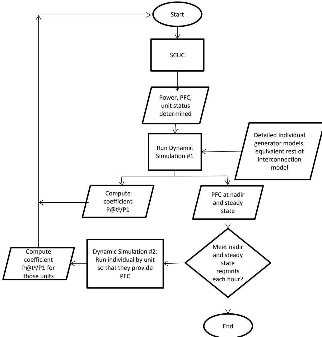
**Figure 2-2. Process for ensuring that PFC is triggered fast enough to avoid UFLS, and that it is fully deployed within a time limit to ensure stability and limit risk.**
