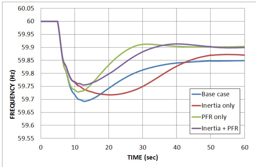
Figure 3-42. WI frequency response for 15% wind power penetration.
