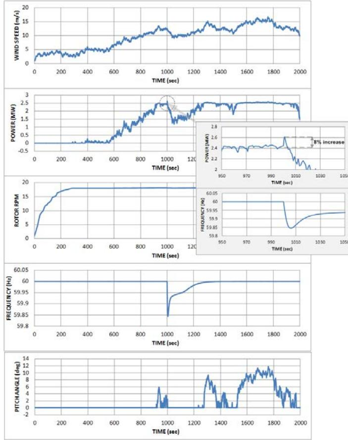
**Figure 3-7. Inertial response of Type 1 WTG during normal operation.**
