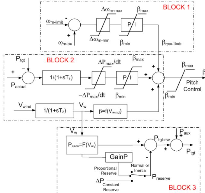
**Figure 3-13. Pitch controller used to set reserve power for Type 1 and Type 2 wind turbines.**
