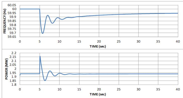
**Figure 3-8. Frequency response for Type 1 WTG connected to a power system with low inertia.**
