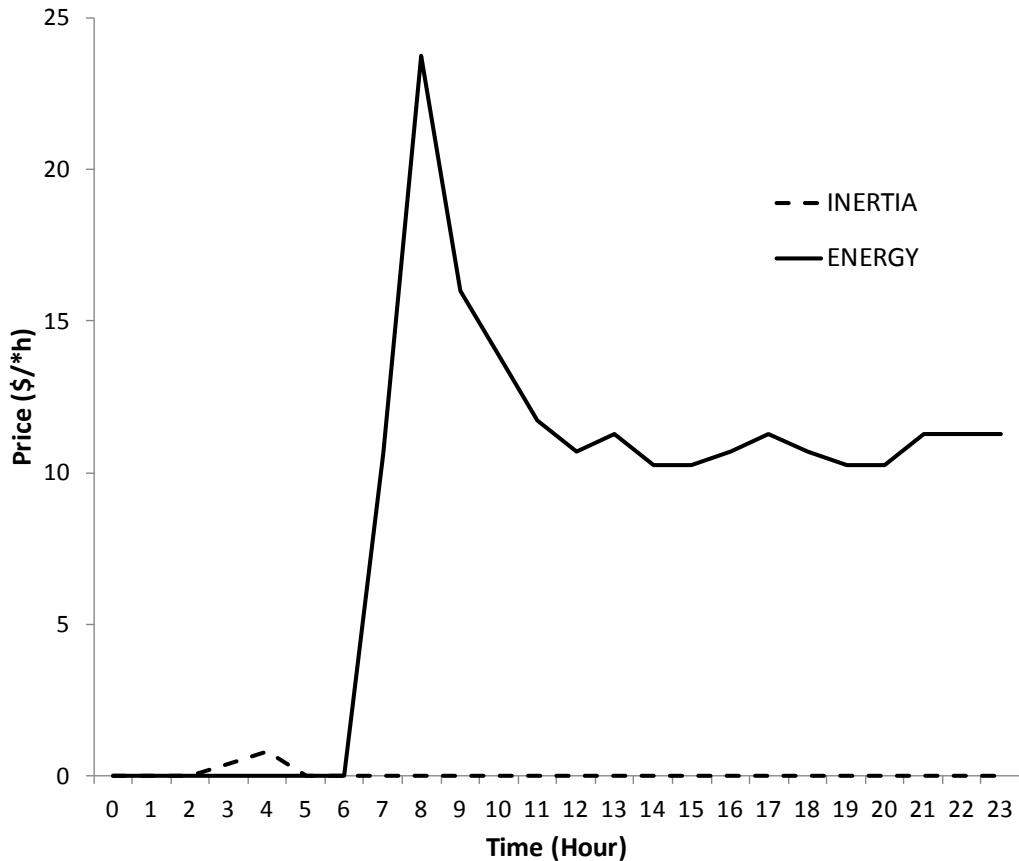
**Figure 2-7. Prices for energy and synchronous inertia for 50% wind penetration system with all other PFC constraints eliminated. Prices are in (\$/MVA-h) for inertia and (\$/MWh) for energy.**
