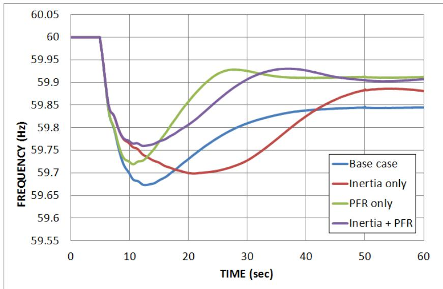
Figure 3-43. WI frequency response for 20% wind power penetration.
