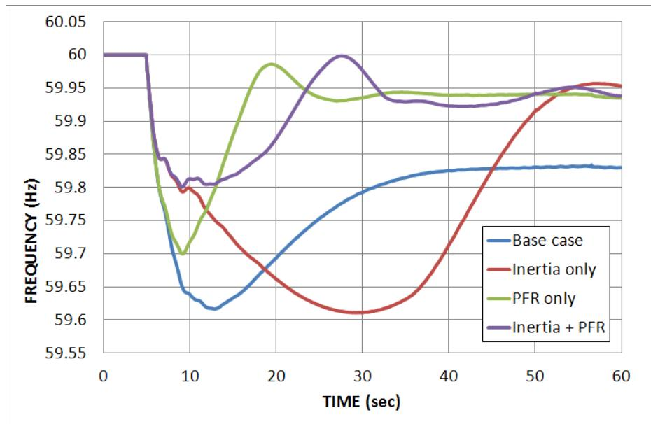
**Figure 3-45.** WI frequency response for 40% wind power penetration.
