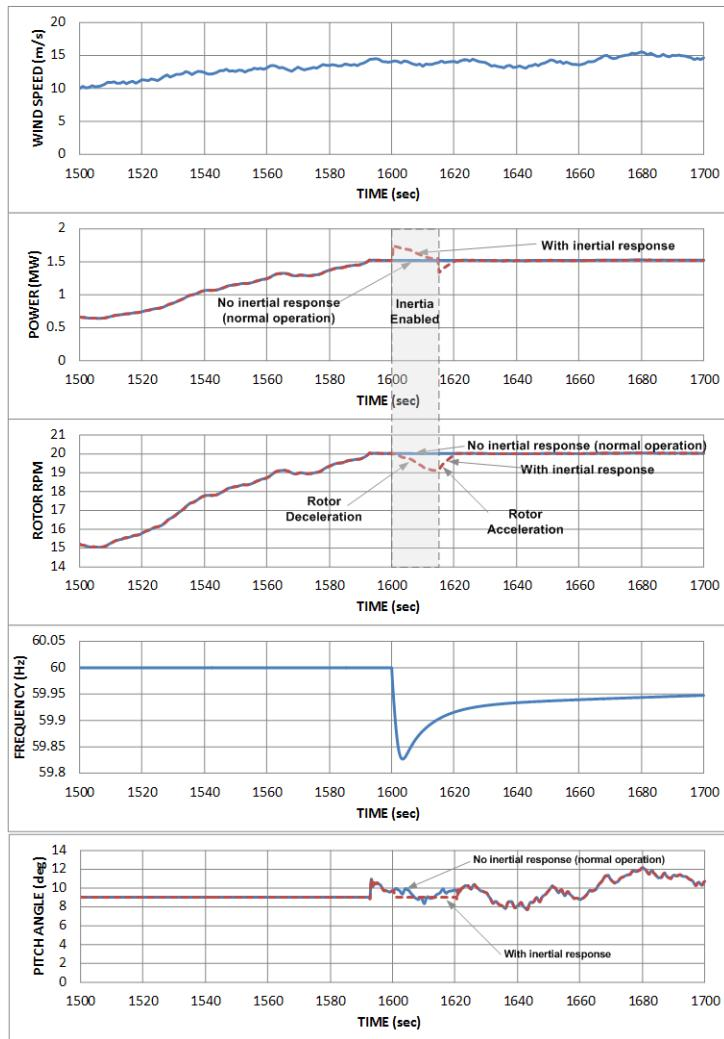
**Figure 3-21. Simulated example of Type 3 inertial control (rated power).**
