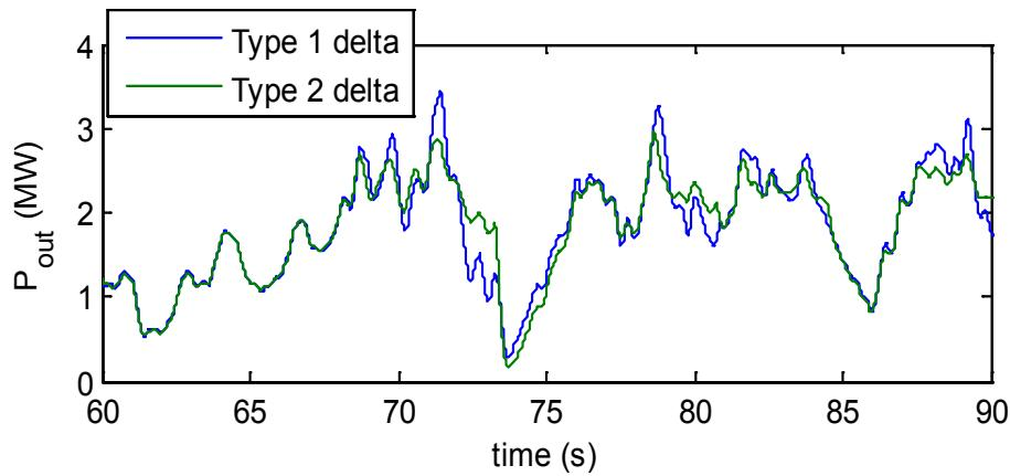
**Figure 3-16.** Output power comparison between the output power of a Type 1 wind turbine and that of a Type 2 wind turbine with  $\Delta P_{\text{reserve}} = 20\%$  of the rated power in time domain.
