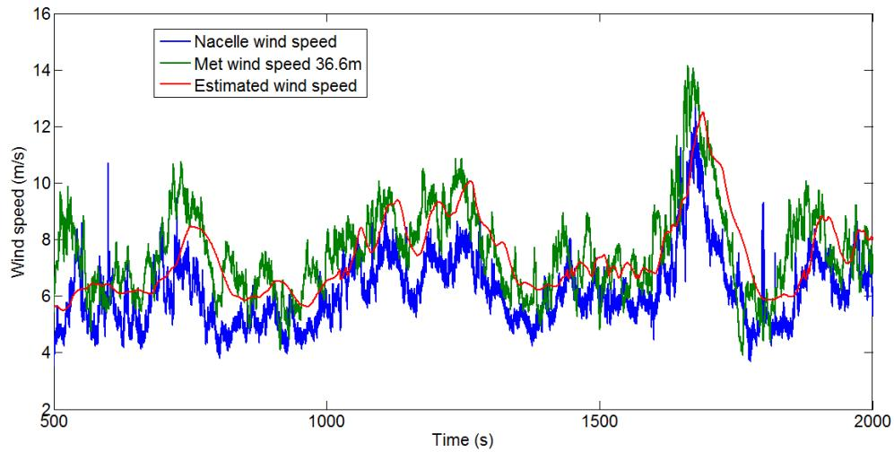
**Figure 4-14. Performance of the wind speed estimator in a field test on the CART3.**
