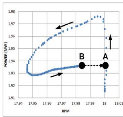
**Figure 3-5. Trajectory of operating point during a frequency decline for Type 1 WTG for a system with large inertia.**
