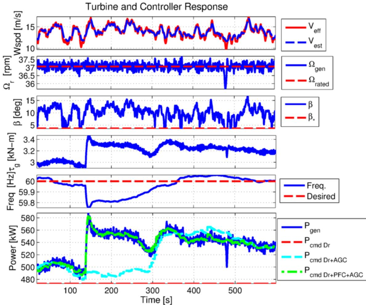
**Figure 4-9.** A simulation of the turbine and control system with above-rated turbulent winds showing AGC and PFC capability. The control system is operating in de-rating mode 1 with de-rating power command of 0.8. The AGC power commands were derived from the ACE that was recorded at a different time than the grid frequency data that was passed into the controller, which uses a 2.5% droop curve to generate the PFC commands.
