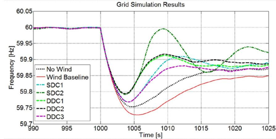
**Figure 4-2. Simulation results from a single bus power system. At  $t = 1000$  s, 5% of generating capacity goes offline. The system response with all conventional generation is compared to the cases when there is a wind plant at 15% penetration without wind plant control or with the droop curve and APC system configurations.**
