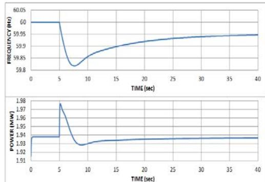
**Figure 3-6. Frequency response of Type 1 WTG connected to a power system with large inertia.**
