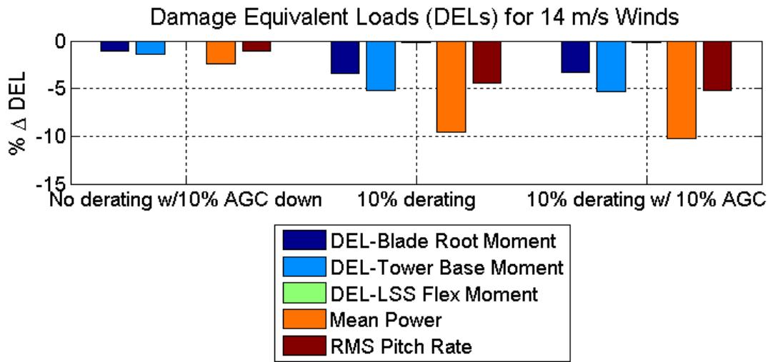
**Figure ES-7. The induced DELs on turbine components comparing de-rating and AGC utilization.**
