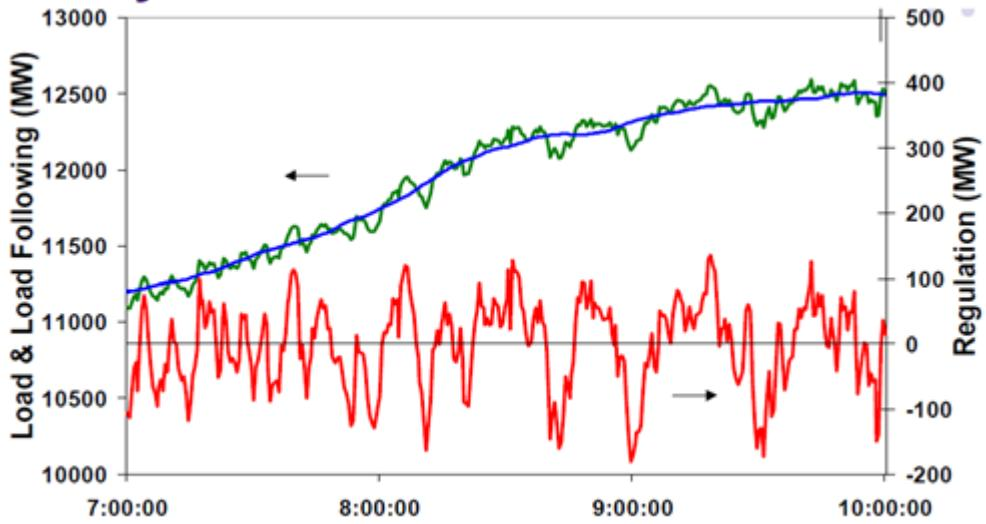
**Figure 1-3. Regulation and load following during normal conditions.**
