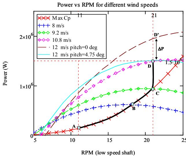
**Figure 3-19. Illustration of kinetic energy transfer during a frequency decline for Type 3 and 4 WTGs.**
