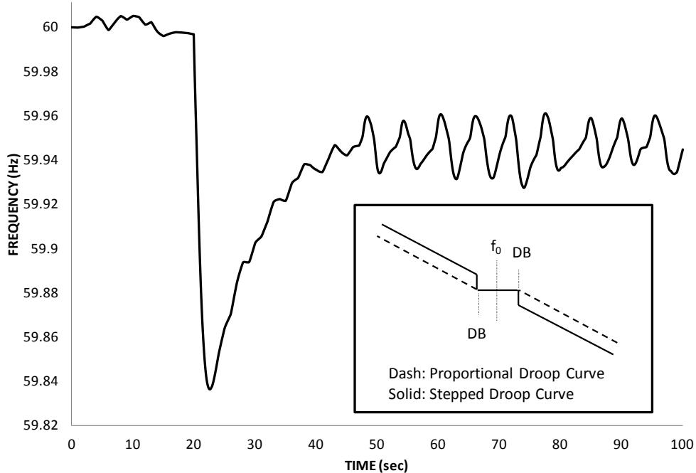
**Figure 2-3. Simulated frequency response following disturbance with units having a stepped droop curve governor response and illustration of proportional vs. stepped droop curves.**
