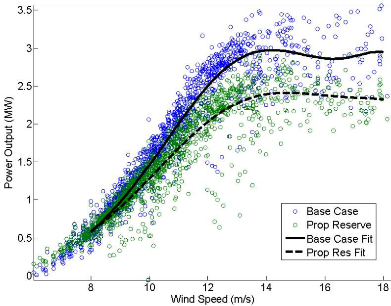
**Figure 3-18. Output power comparison between the base case and proportional reserve power of a Type 2 wind turbine based on the dynamic simulation with  $\Delta P_{\text{reserve}} = 20\%$  of the rated power.**
