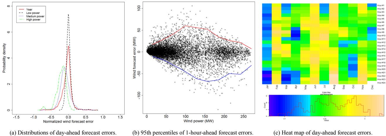
Figure 5. Analysis of wind forecast errors of the power system in Norway.
