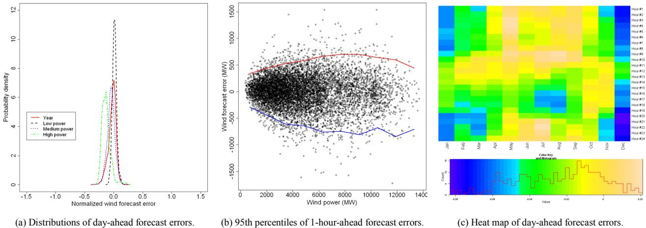
Figure 3. Analysis of wind forecast errors of the power system in Spain.
