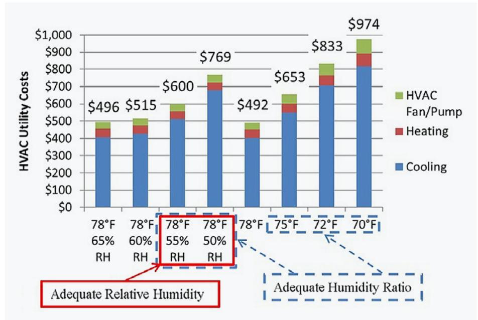
CARB used NREL’s BEOpt energy simulation software to analyze the cost effectiveness of various cooling system configurations.
