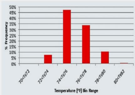
Indoor temperature was maintained within comfortable limits of 74°F to 80°F for 91.5% of the monitoring period. Excluding the sub-74°F indoor conditions (lower than cooling set point temperature), the home was kept within the comfort zone temperature range for 99.3% of the cooling portion of the monitored period.
