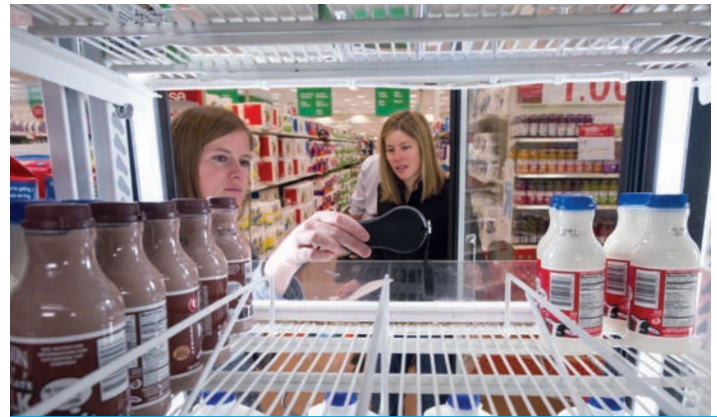
NREL engineers check light levels in a refrigerated display case at a Target store, to compare the performance of LED and fluorescent case lights. Photo by Dennis Schroeder, NREL19510
