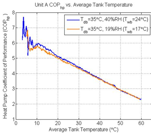
**Figure 11. Effect of humidity on COP<sub>hp</sub> for Unit A**
