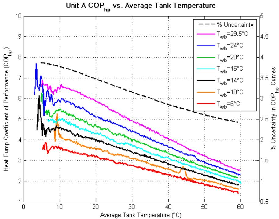
**Figure 10. COP<sub>hp</sub> traces for Unit A**
