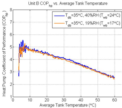
**Figure 17. Effect of humidity on COP<sub>hp</sub> for Unit B**
