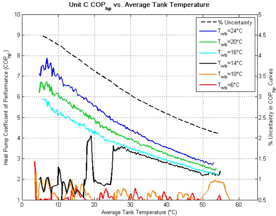
**Figure 22. COP<sub>hp</sub> traces for Unit C**
