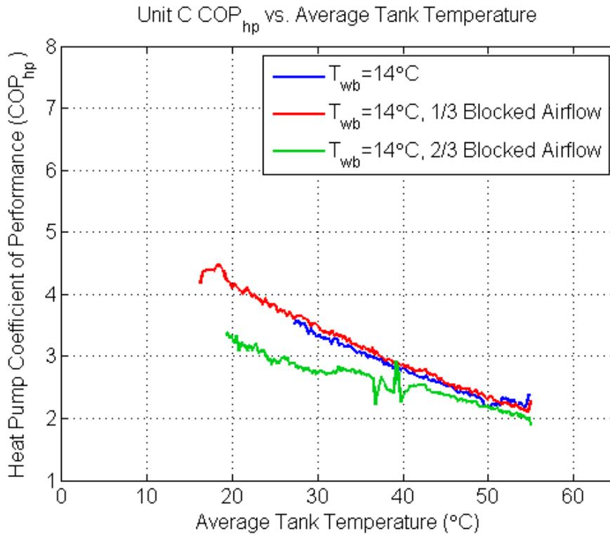
**Figure 25. COP<sub>hp</sub> traces for Unit C with reduced airflow**
