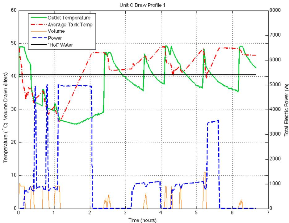
**Figure 21. Draw Profile 1 for Unit C**
