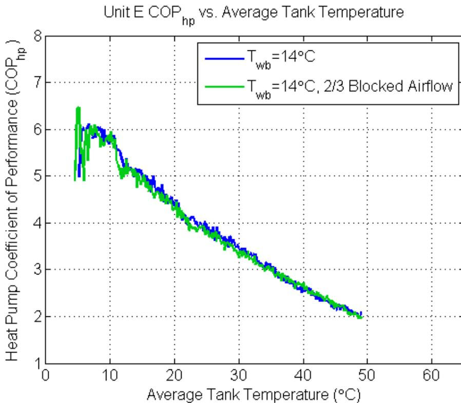
Figure 37. COP<sub>hp</sub> traces Unit E with reduced airflow
