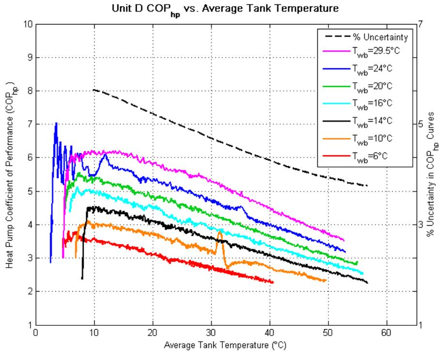
**Figure 28. COP<sub>hp</sub> traces for Unit D**
