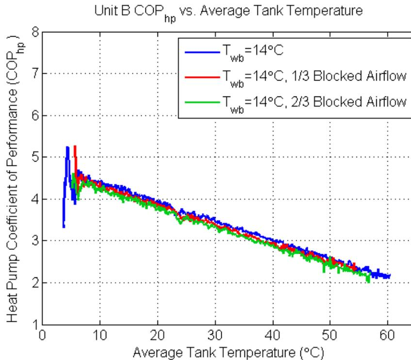
**Figure 19. COP<sub>hp</sub> traces for Unit B with reduced airflow**
