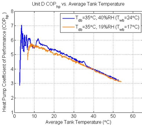
Figure 29. Effect of humidity on COP<sub>hp</sub> for Unit D
