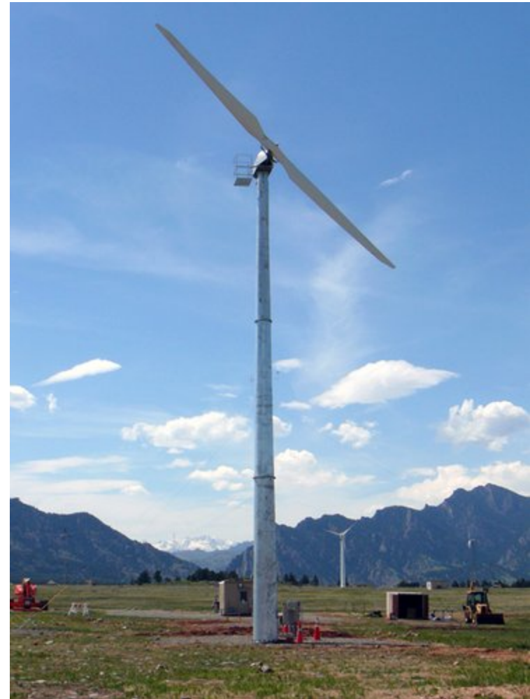
An 11-kW Gaia small wind turbine. Photo by Lee Jay Fingersh, NREL 17523
