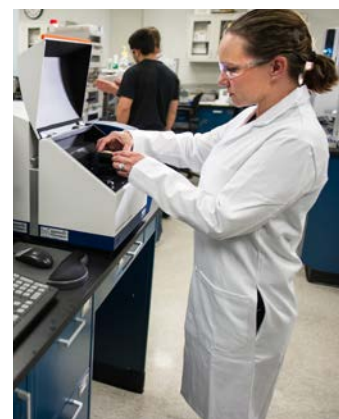
An NREL researcher scanning solid biomass samples for rapid near-infrared (NIR) compositional analysis based on chemometric models. NREL 26487.
