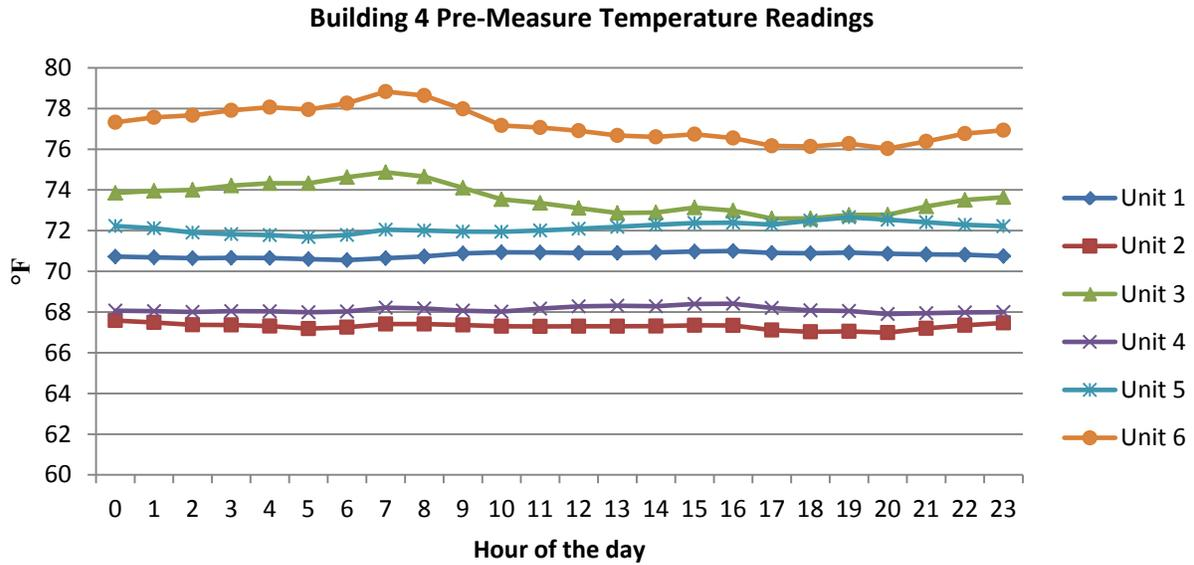
**Figure 11. Building 4 average pre-measure logging period temperature readings by hour of the day**
