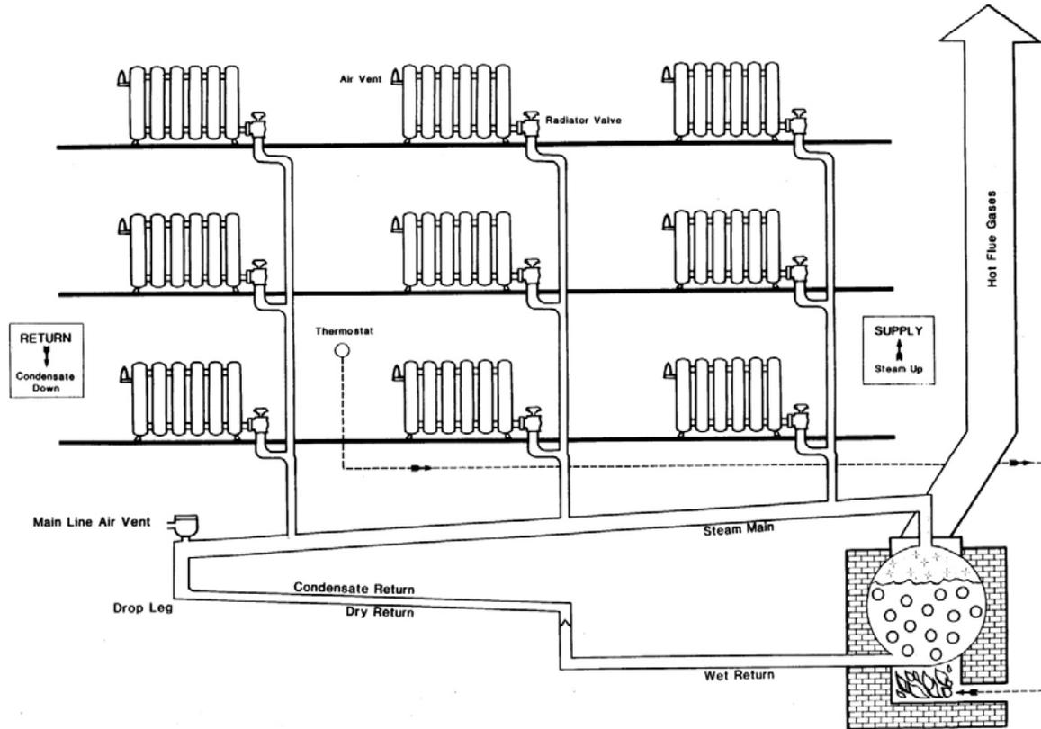
**Figure 1. Schematic of single-pipe steam system**
