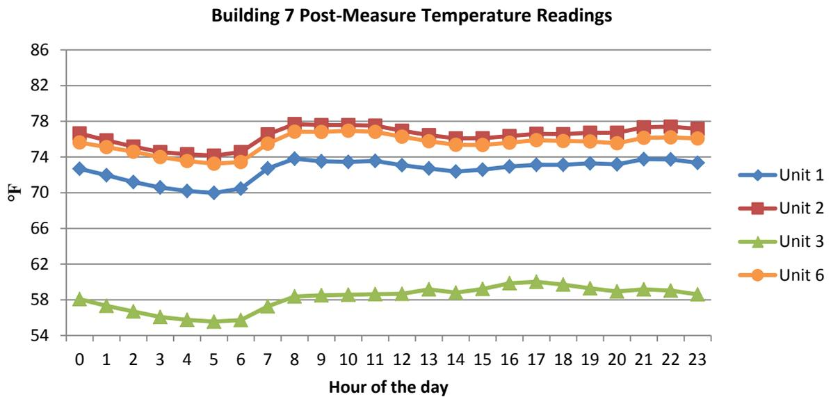
Note: Post-measure data for Units 4 and 5 were unavailable because of limited access to the units. The logger for Unit 3 had been moved from where it was installed to the floor and therefore showed very low temperatures.
