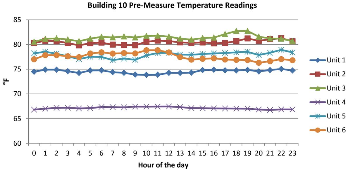
**Figure 9. Building 10 average pre-measure logging period temperature readings by hour of the day**
