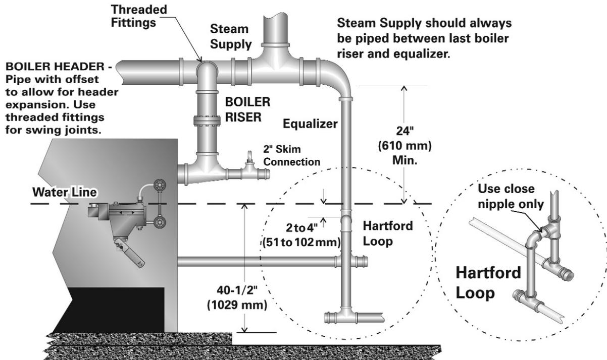
**Figure 5. Specifications for how to pipe a Series 211A™ natural gas steam boiler by Peerless®**
