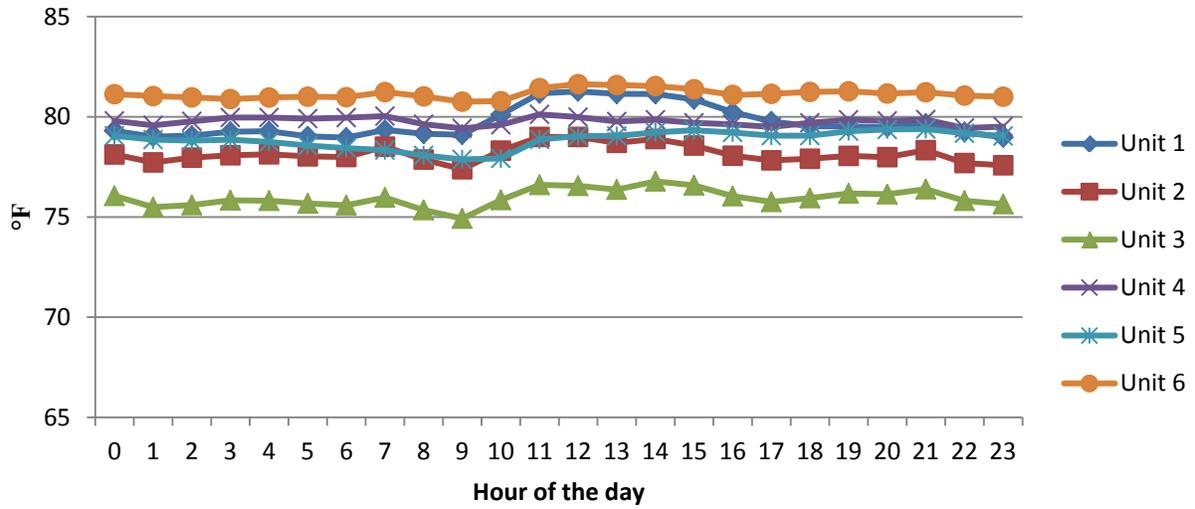
**Building 3 Post-Measure Temperature Readings**
