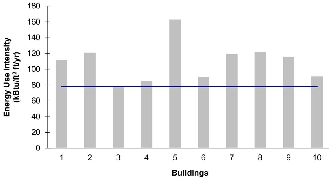
**Figure 17. The pre-measure heating EUI for each test building is at or above the line representing the median EUI for 105 similar steam-heated buildings in Chicago. This suggests that the buildings chosen for this study all had potential for energy savings.**
