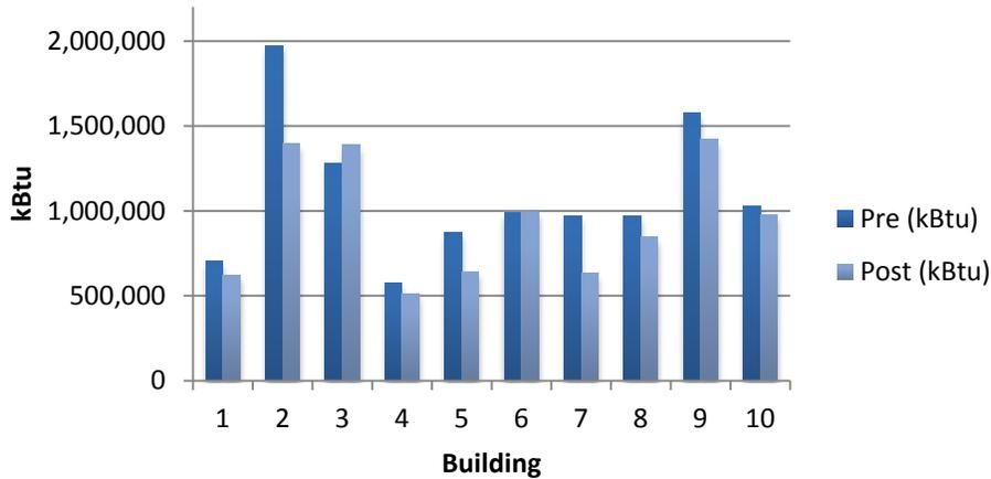
Figure 13. Weather-normalized natural gas use from utility bills during pre-balancing and post-balancing periods
