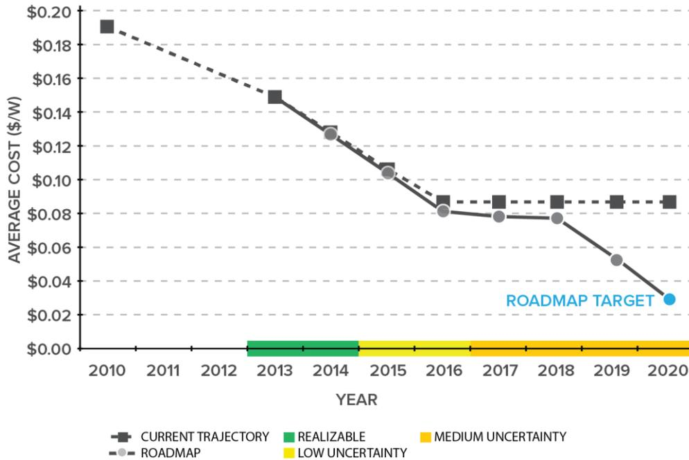
Figure 5. Commercial PV customer acquisition costs: Current trajectory and roadmap
