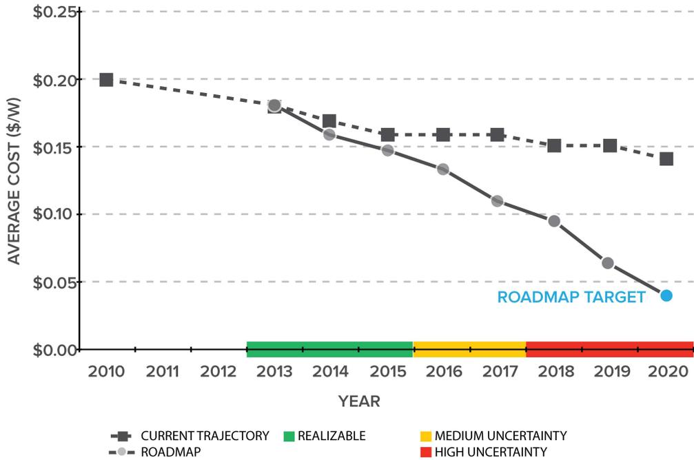
**Figure 7. Residential PV permitting, inspection, and interconnection costs: Current trajectory and roadmap**
