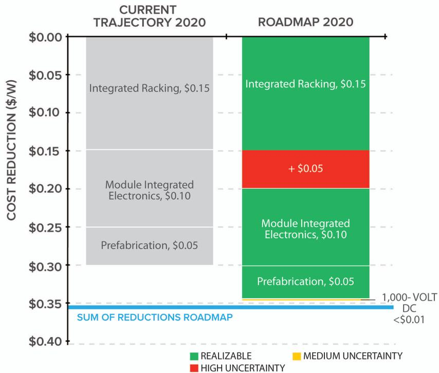
Figure 12. 2020 commercial PV installation labor cost reductions: Current trajectory and roadmap
