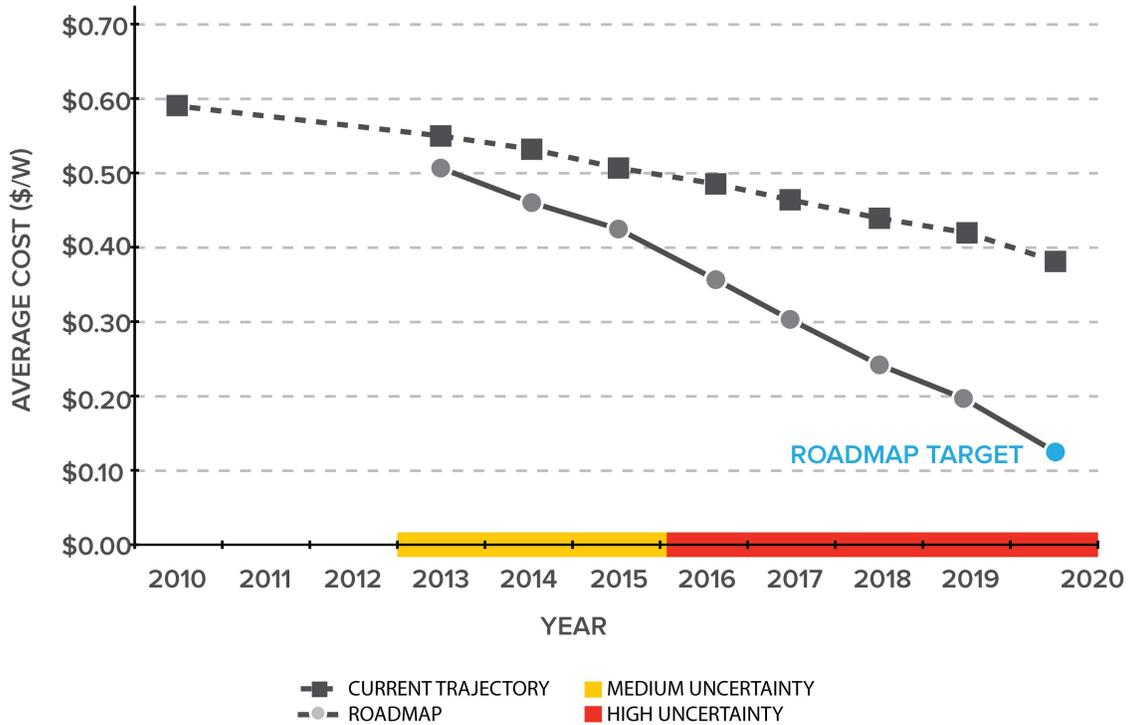
Figure 9. Residential PV installation labor costs: Current trajectory and roadmap
