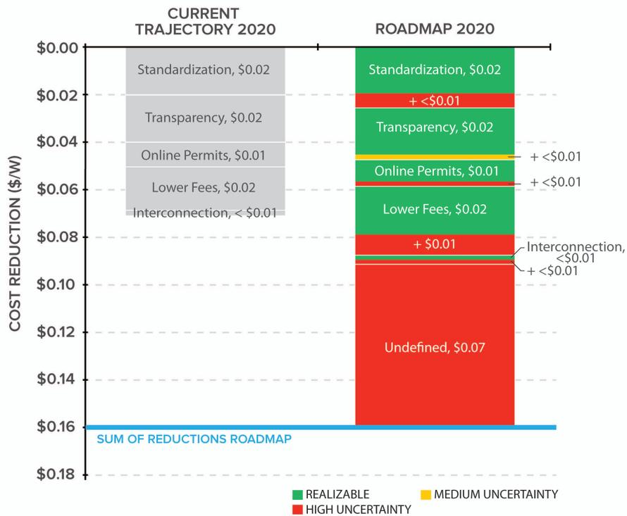
**Figure 8. 2020 residential PV permitting, inspection, and interconnection cost reductions: Current trajectory and roadmap**
