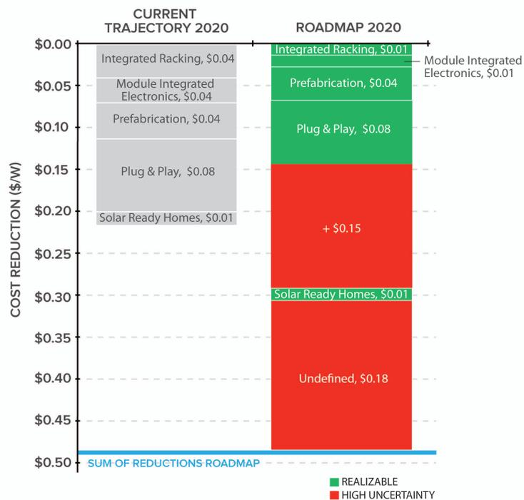
Figure 10. 2020 residential PV installation labor cost reductions: Current trajectory and roadmap
