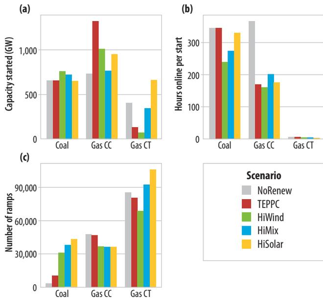
**Figure 1.** (a) Capacity started, (b) average number of hours online per start (must-run CTs were excluded), and (c) total number of ramps for each plant type by scenario for one year
