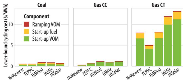
**Figure 2.** Lower-bound cycling cost for (left) coal, (center) gas CC units, and (right) gas CTs (excluding the must-run CTs) for one year
