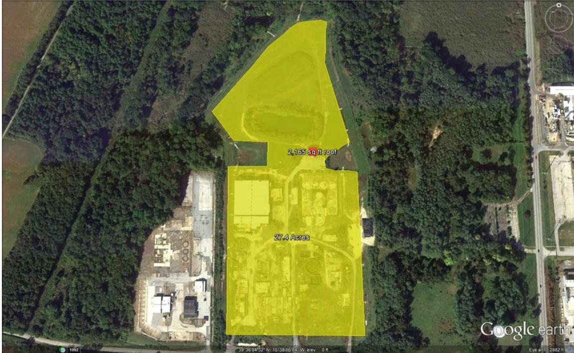
**Figure 6. Aerial view of the feasible areas for PV at the Standard Chlorine of Delaware site (ground-mounted PV in yellow and treatment system building with roof-mounted PV in red)**
