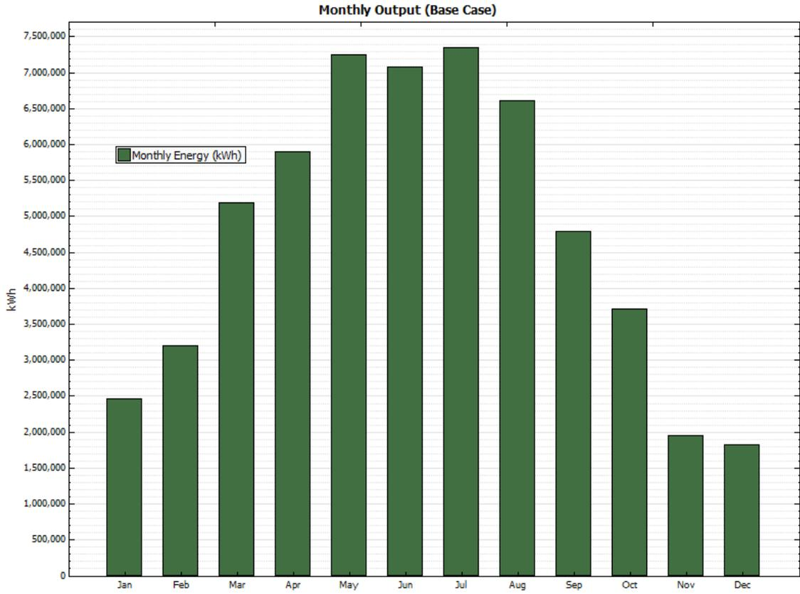
**Figure B-9. Monthly energy output—Industrial (red shaded) area—Single axis—40,948 kW**
