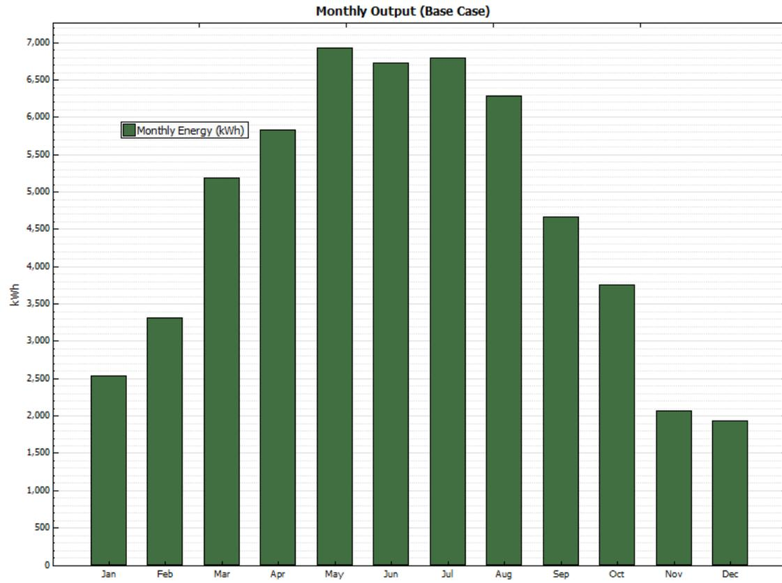
**Figure B-37. Monthly energy output—Capacity-based incentive limit—Fixed axis—50 kW**
