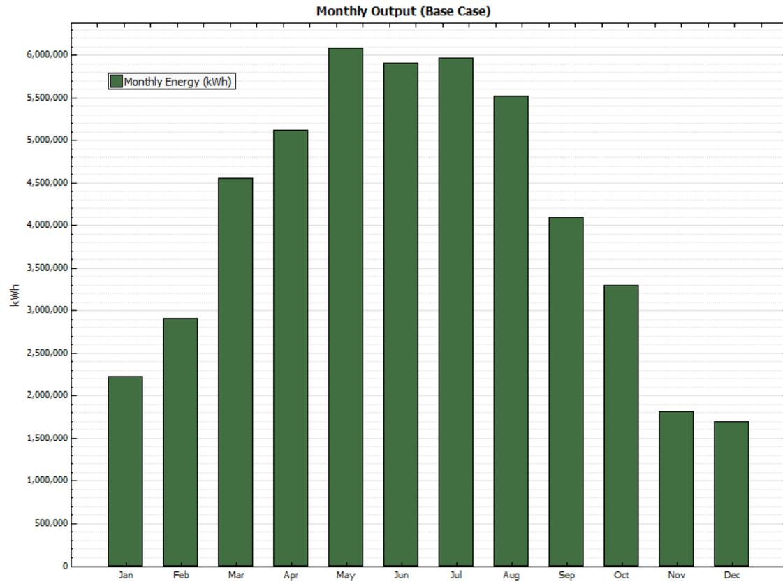
**Figure B-6. Monthly energy output—Primary (yellow shaded) area—Fixed axis—43,902 kW**
