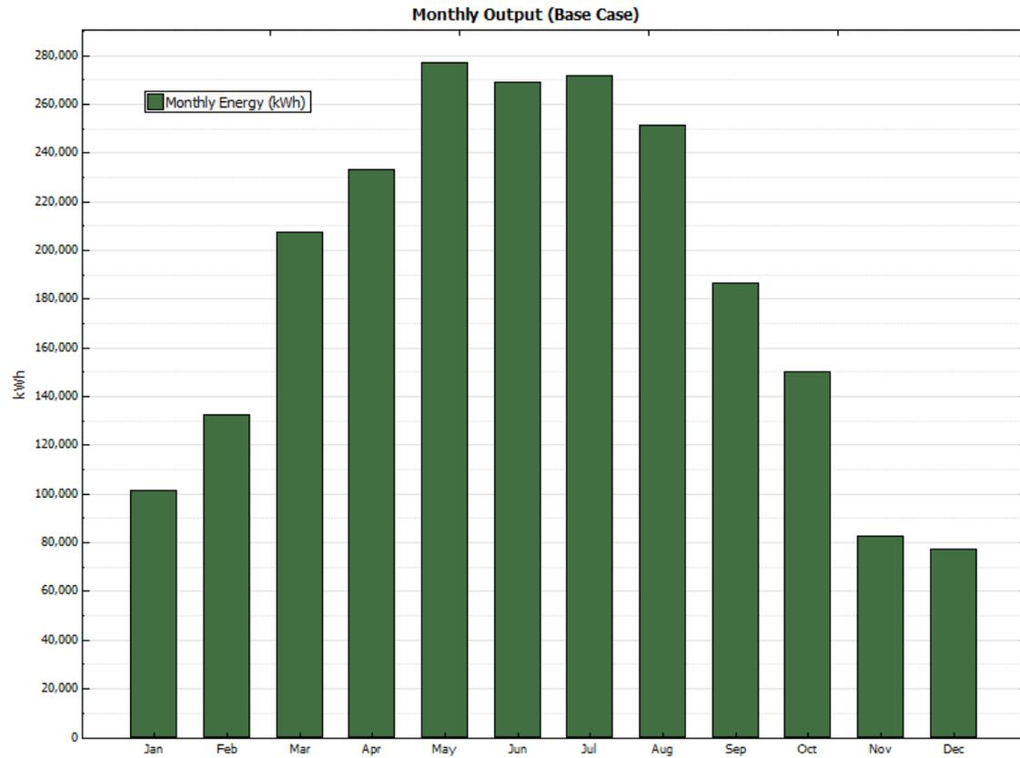
**Figure B-31. Monthly energy output—Net-metering limit—Fixed axis—2,000 kW**
