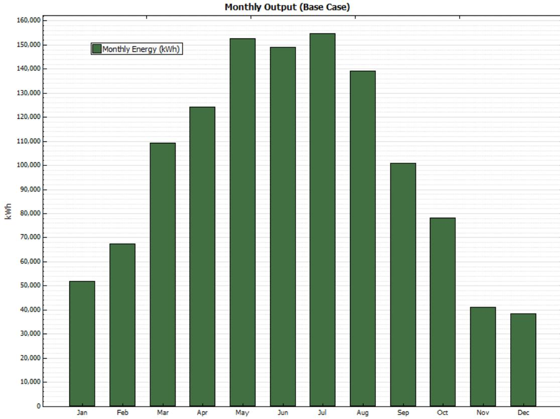
**Figure B-40. Monthly energy output—Largest system with positive NPV—Fixed axis—862 kW**
