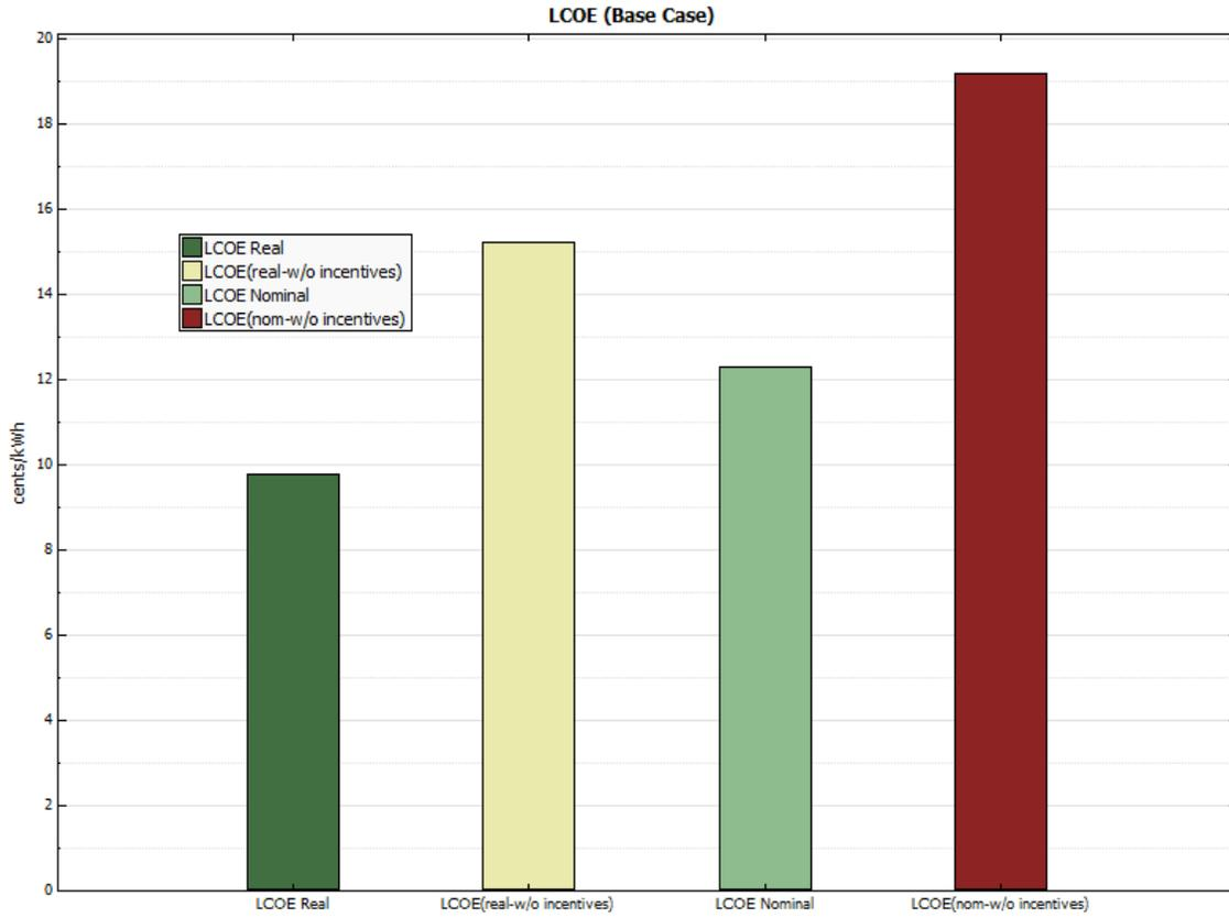
**Figure B-20. Levelized cost of energy—Highly contaminated (purple shaded) area—Single axis—9,626 kW**
