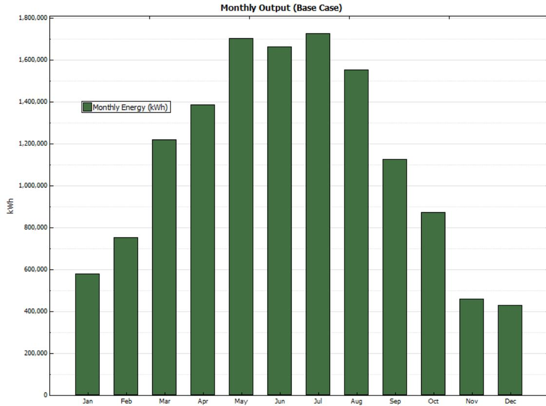
**Figure B-22. Monthly energy output—Highly contaminated (purple shaded) area—Single axis—9,626 kW**
