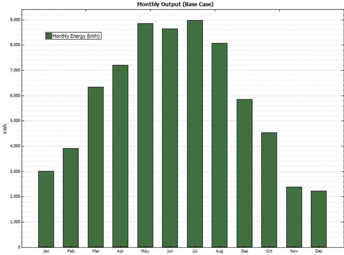
**Figure B-34. Monthly energy output—Capacity-based incentive limit—Single axis—50 kW**
