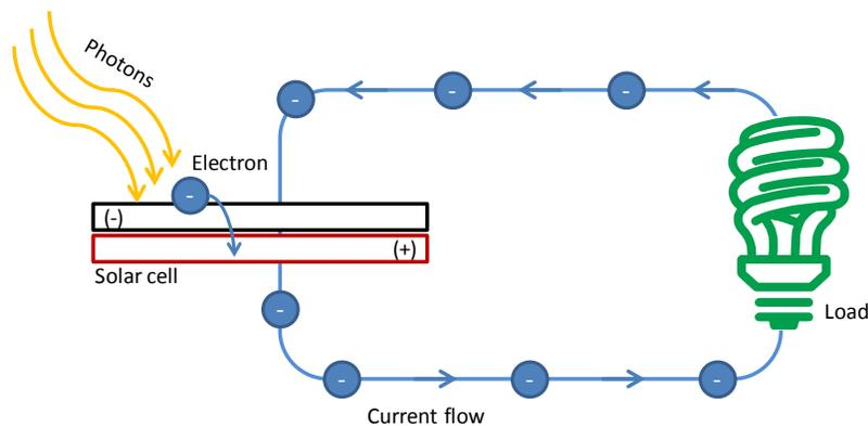
**Figure 1. Generation of electricity from a PV cell**
