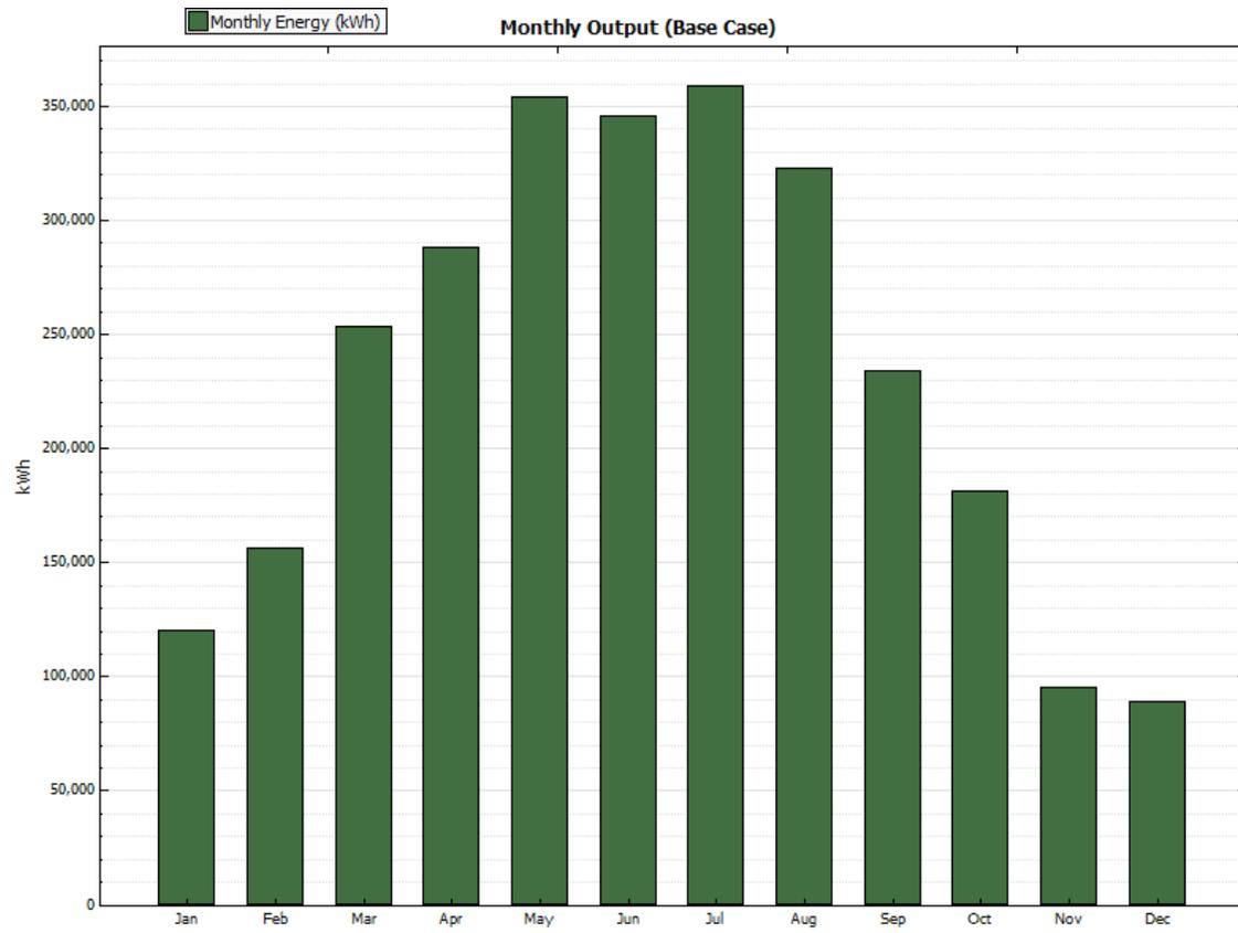
**Figure B-28. Monthly energy output—Net-metering limit—Single axis—2,000 kW**
