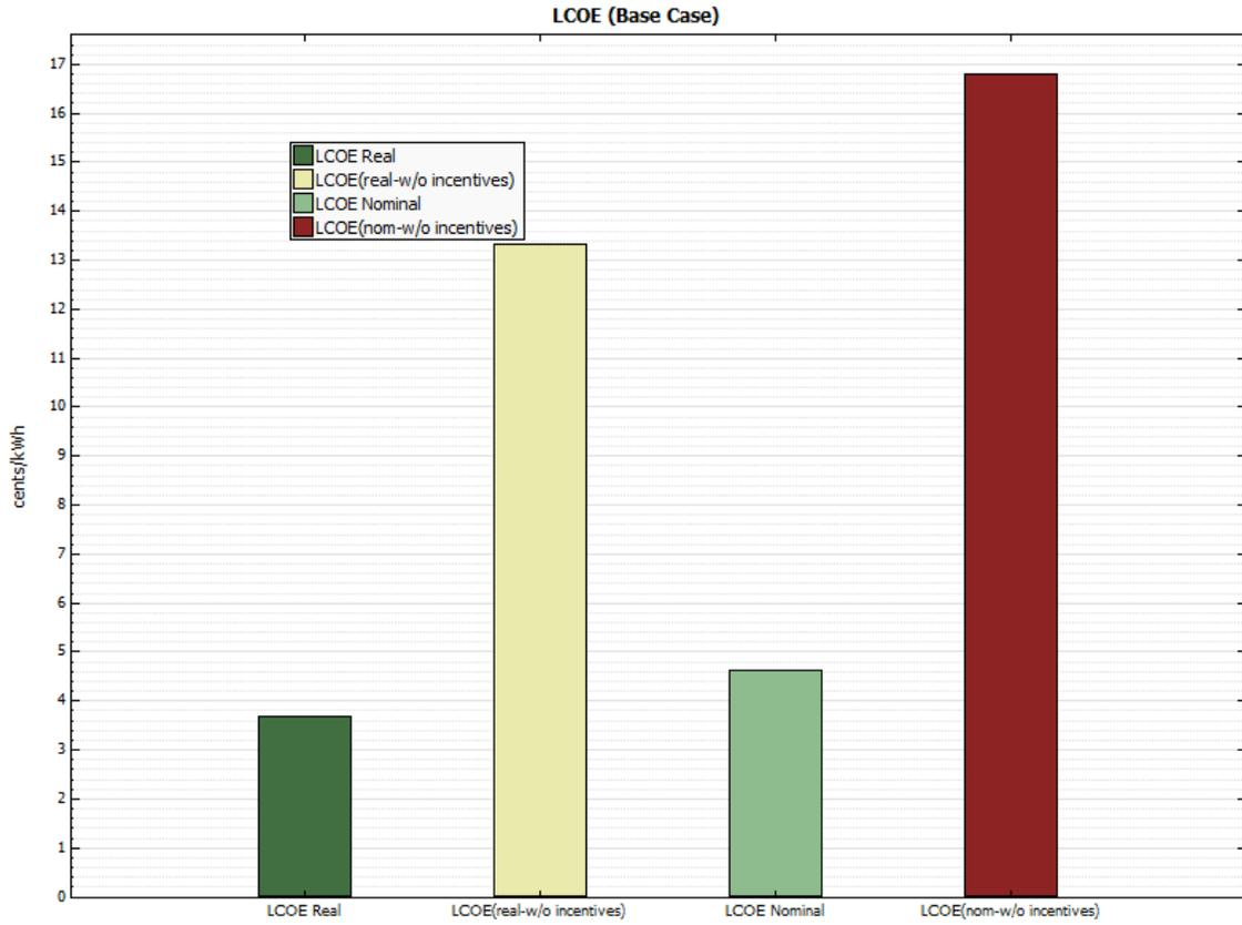
Figure B-35. Levelized cost of energy—Capacity-based incentive limit—Fixed axis—50 kW
