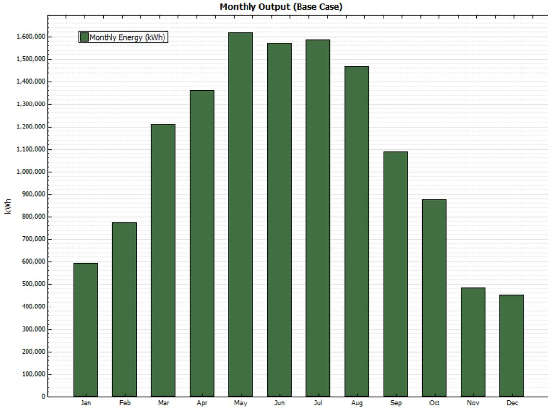
**Figure B-25. Monthly energy output—Highly contaminated (purple shaded) area—Fixed axis—11,672 kW**
