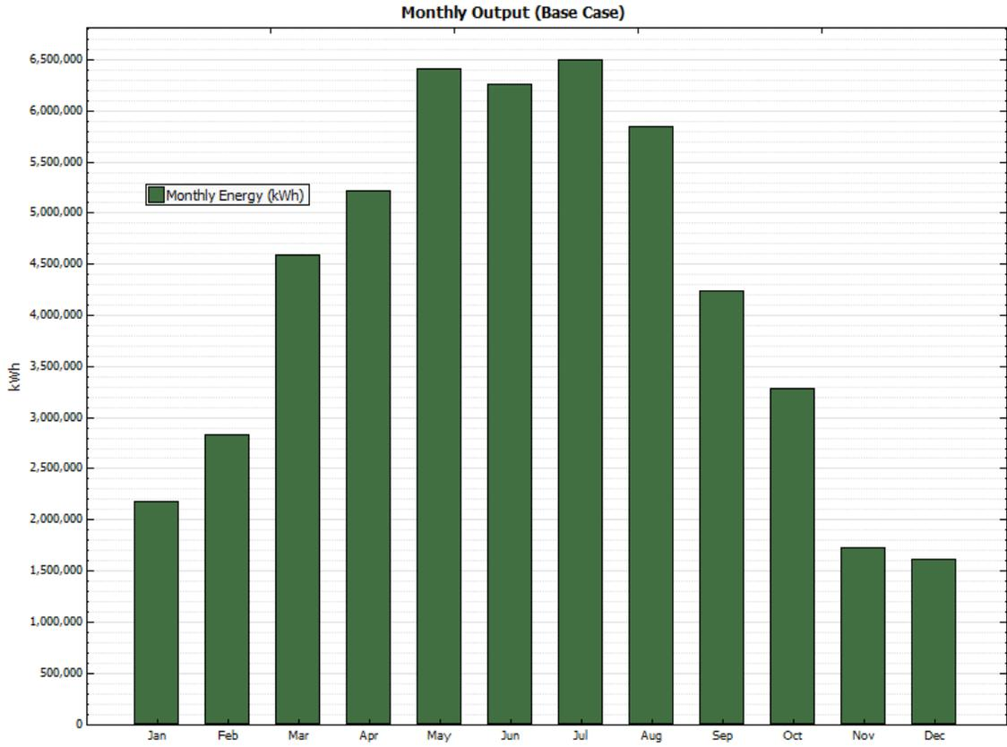
**Figure B-3. Monthly energy output—Primary (yellow shaded) area—Single axis—36,206 kW**
