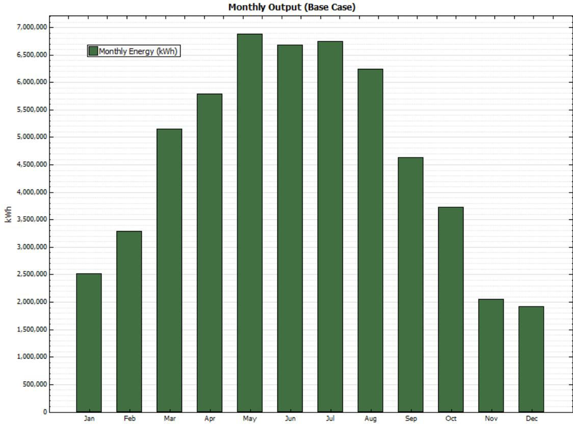
**Figure B-12. Monthly energy output—Industrial (red shaded) area—Fixed axis—49,651 kW**
