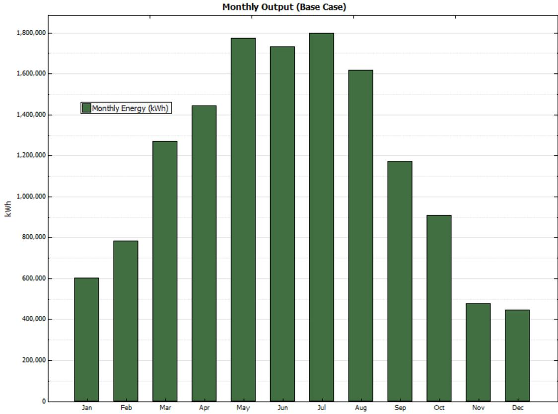
**Figure B-16. Monthly energy output—Wind turbine (green shaded) area—Single axis—
