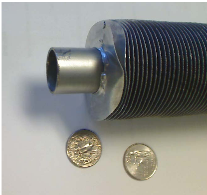
Figure 1. A photograph of a typical ACC tube with fins. Photo by Desikan Bharathan, NREL 24524.
