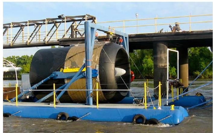
Hydrokinetic turbine generator deployed on a floating mount in the Mississippi River. *Photo from Free Flow Power Corp*
