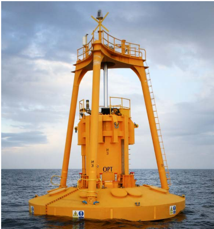
Ocean Power Technologies' PowerBuoy, currently being tested off the Oregon coast, generates power from ocean waves without polluting.
