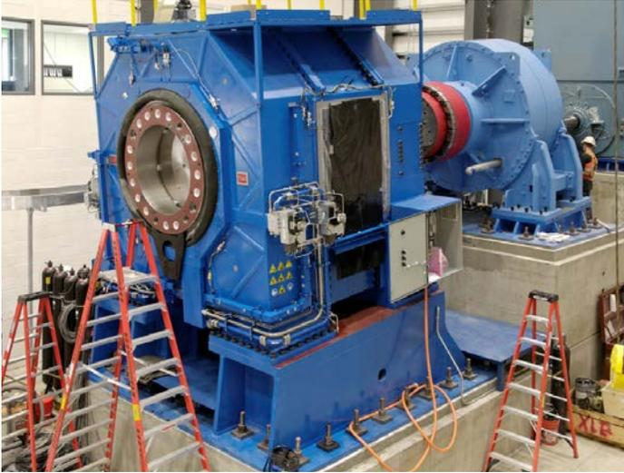
NREL's National Wind Technology Center will house one of the largest dynamometers in the world, which will help accelerate wind technology development by enabling testing of the performance and reliability of both wind turbine drivetrain prototypes and commercial machines with capacity ratings up to 5 megawatts.
