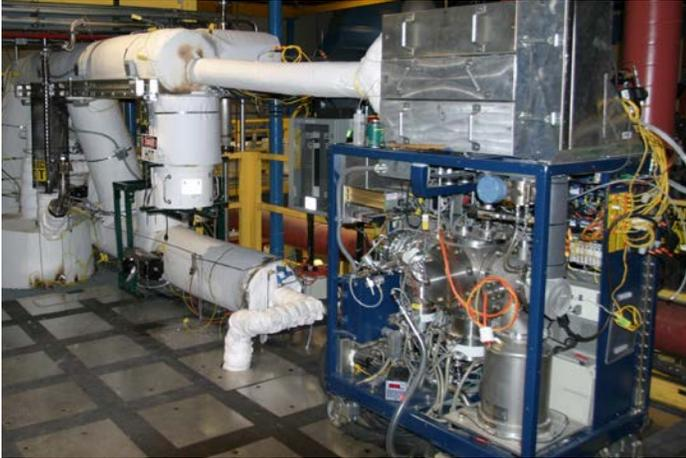
NREL installed a Molecular Beam Mass Spectrometer—a scientific measuring device that allows real-time, detailed analysis of gaseous vapors. *Photo by Calvin Feik, NREL 16021*
