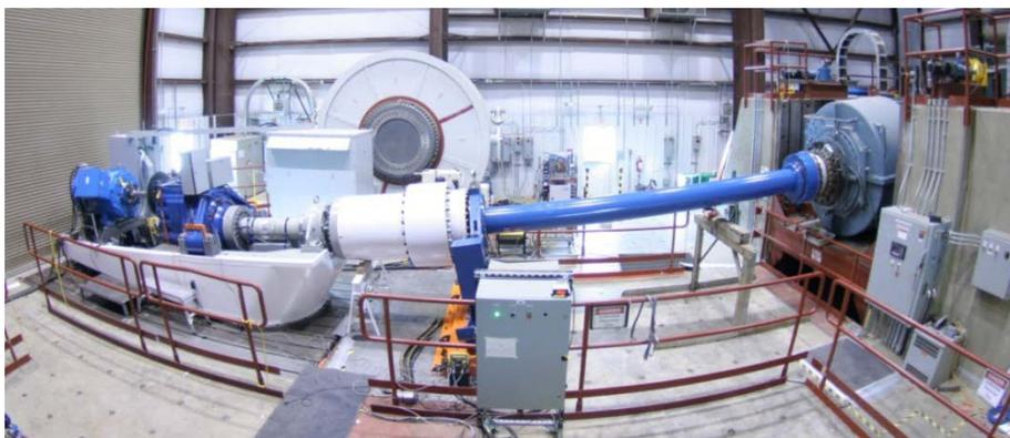
Figure 6: NREL dynamometer test stand with 750-kW gearbox article installed. Photo by Lee Jay Fingersh / NREL 16913.
