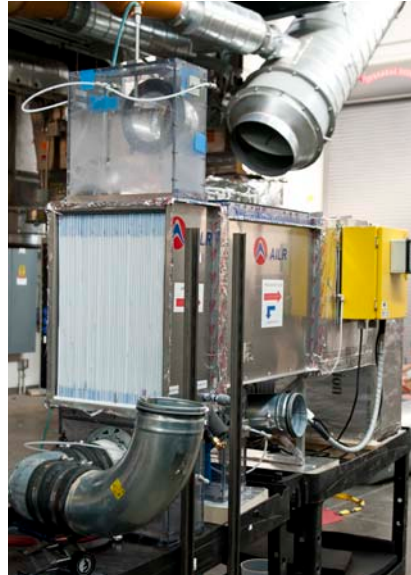
A DEVAP prototype undergoing testing at the Advanced HVAC Systems Laboratory. Photo by Dennis Schroeder, NREL 20200
