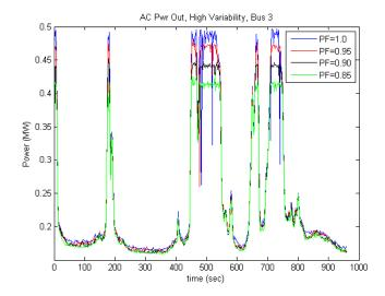
(b) PV inverter real power output for PF set-points of 1.0, 0.95, 0.9, and 0.85 for the high PV array power ouput variability case
