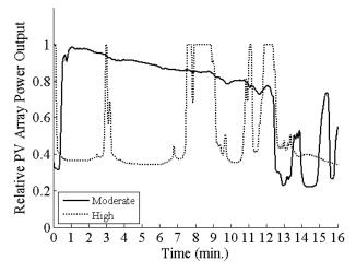
Fig. 2. Relative PV array power output profiles used during PHIL testing based on normalized moderate and high PV array irradiance profiles.
