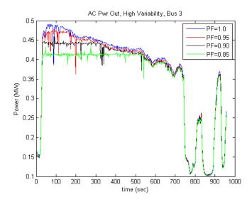
(a) PV inverter real power output for PF set-points of 1.0, 0.95, 0.9, and 0.85 for the moderate PV array power ouput variability case
