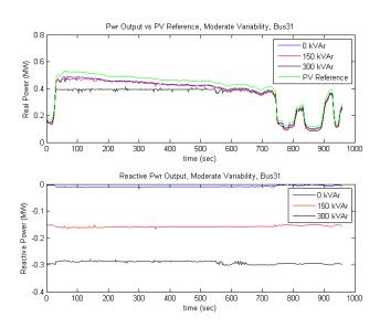
Fig. 7. Plots of the PV inverter real power output (top) and reactive power output (bottom) during PHIL simulation runs for moderate and high PV array power variability
