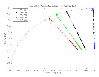
(b) X-Y plot of the real and reactive power during 16 minute real-time PHIL simulations for constant PF control mode set-points of 1.0, 0.95, 0.90, and 0.85 for the high PV array power varaibility case
