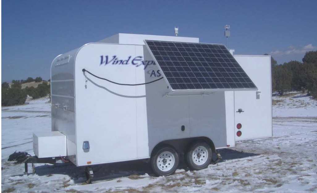
Figure 6. The Wind Explorer™ miniSODAR unit from Atmospheric Systems Corporation Photo credit: Robi Robichaud, NREL
