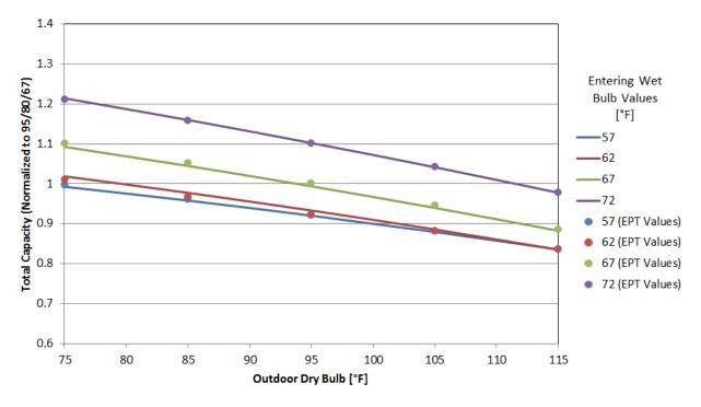
Figure 2. Comparison of total capacity performance curve to manufacturer EPT values
