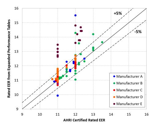
**Figure 6. Comparison of AHRI-certified EER to manufacturer EPT data for single-stage ACs** The equation to calculate SEER for single-stage equipment is
