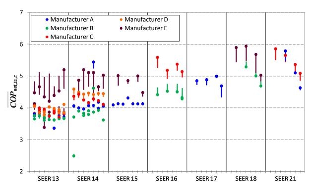
Figure 5. Variations in simulation results attributed to using a fixed set of performance curves (individual capacities of 1.5, 2, 3, 4, and 5 tons shown in ascending order within SEER values)
