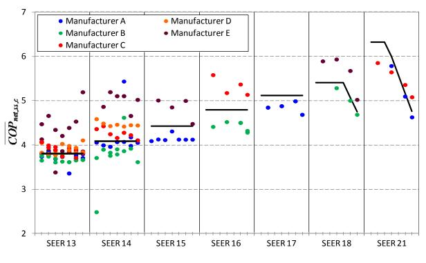
Figure 10. Simulation results for the AC library (shown in solid black lines) compared to individual AC units (individual capacities of 1.5, 2, 3, 4, and 5 tons shown in ascending order within SEER values)
