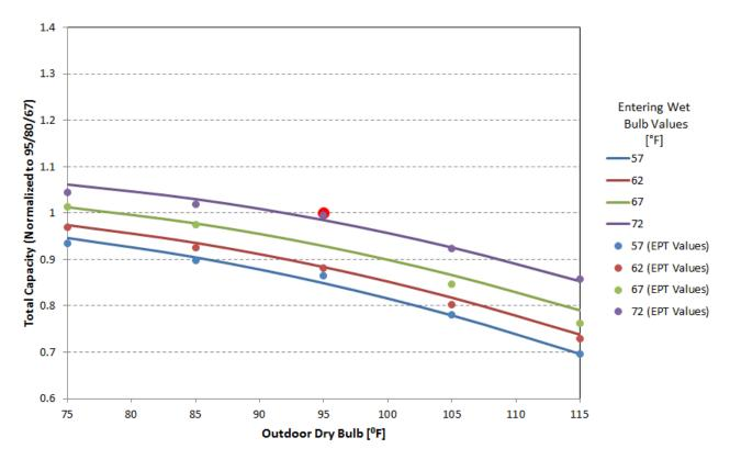
Figure 3. Comparison of total capacity curve to manufacturer data with an adjusted rating point (shown in red)
