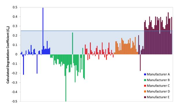
Figure 7. Back-calculated  $C_{\rm D}$  values for single-stage ACs using AHRI SEER values and manufacturer EPT data
