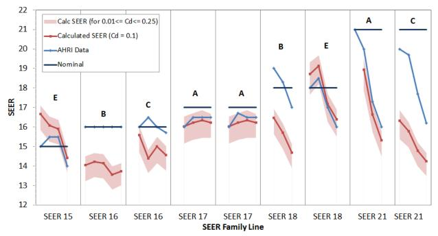
Figure 9. SEER calculated using manufacturer data compared to AHRI reported SEER values for two-stage ACs (letters A, B, C, and E denote manufacturer; capacities of 2, 3, 4, and 5 tons shown in ascending order within a product line)
