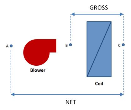
Figure 1. Net versus gross capacity for a blow-through fan configuration
