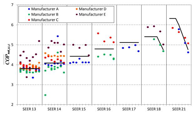
Figure ES–1. Simulation results comparing annual average efficiency of a standard AC component library (shown in black lines) to specific AC units for five leading manufacturers
