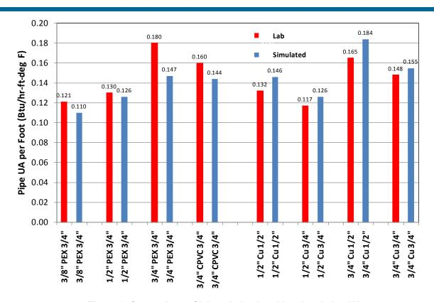
Figure 3. Comparison of lab and simulated insulated pipe UAs
