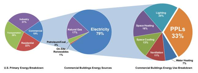
Figure 1. PPLs account for 33% of the total energy consumed by commercial buildings. Graph by Chad Lobato, NREL; Data source: DOE (2010)
