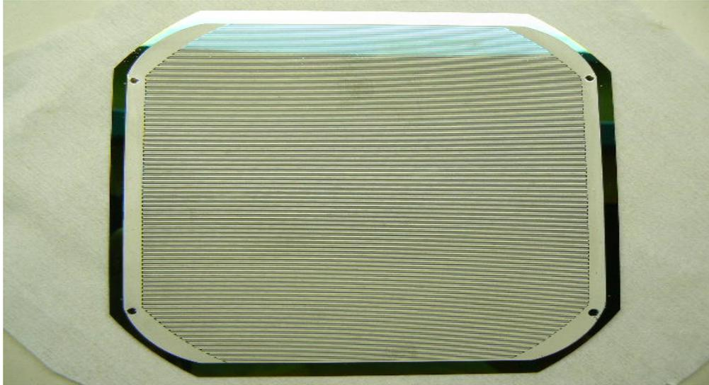
**Figure 14. Backside of a TFSS cell. The emitter and base busbars are located at the edges with interdigitated fingers collecting the current.**
