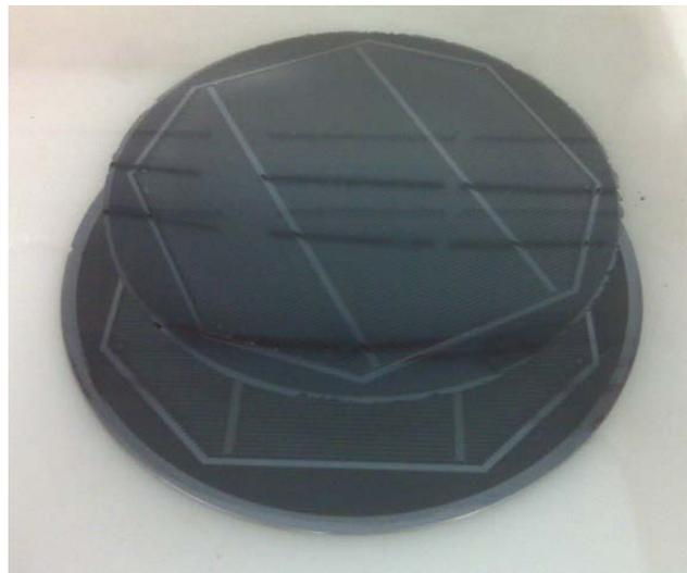
**Figure 3. First 156mmx156mm epitaxial substrate and its master template released using SMR technique.**
