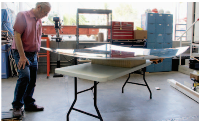
Principal investigator Dr. Roger Angel evaluates a self-supporting second-surface glass reflector made by the new molding process. Photo by The University of Arizona
