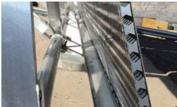
3M is producing high-flux, lightweight reflectors with lightweight, high-precision panels combined with unique multilayer optical film technology. Photo from 3M Company
