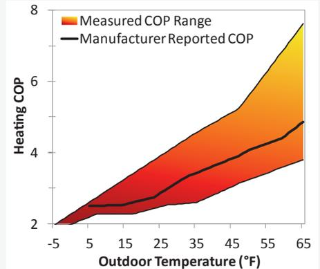
Chart of MSHP heating efficiency (COP) at various outdoor temperatures. The wide colored band represents efficiency variation due to different heating loads. The manufacturer's reported efficiency is indicated by the thick blue line.
