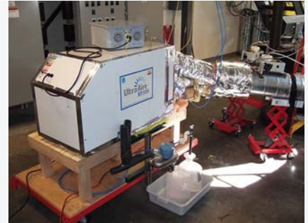
Experimental test setup of the Ultra-Aire XT150H residential dehumidifier in NREL's Advanced HVAC lab in the Thermal Test Facility. Photo by Dane Christensen, NREL/PIX 19601
