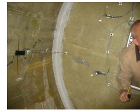
Figure 7. Blade root strain instrumentation.
