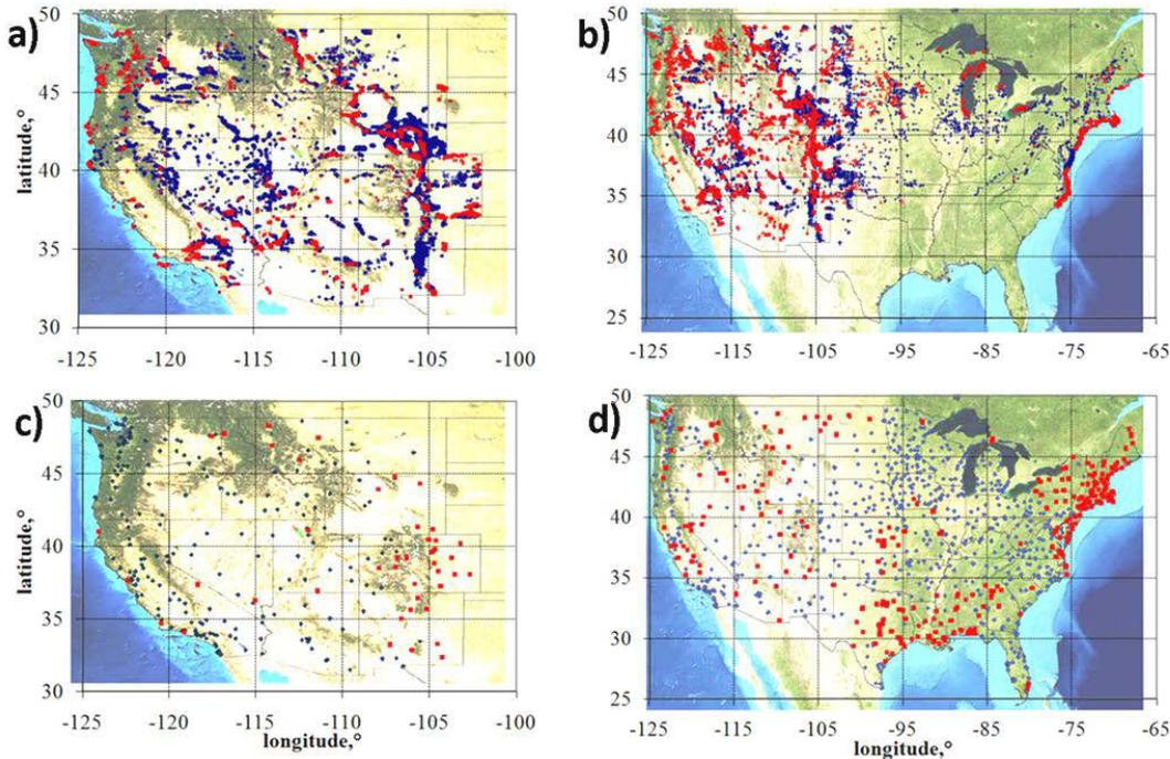
Figure 3. Load matching with dispatchables, wind (a, b) and PV (c, d) buildout for WECC (a, c) and U.S. (b, d). The generation sites that contribute to the optimal solution are shown in red, the remaining sites are shown in blue.
