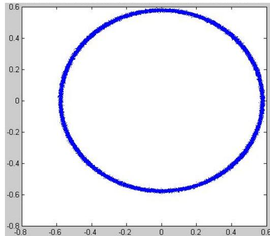
Figure 4. Equidistant projection of pyramid base edge-points on an arbitrarily selected plane. 60,000 randomly selected edge-points are shown.
