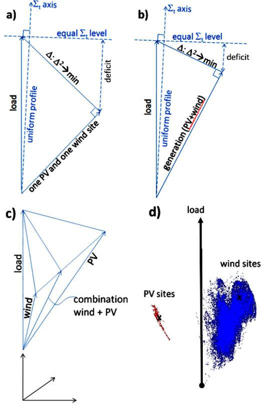
Figure 1 ([7]). Quadratic load matching diagram for the case when a) all generation is concentrated at one PV and one wind site and b) the PV and wind generation sites are selected from all available Western U.S. sites; c) Schematic representation of a three-dimensional diagram shows the combination of wind and PV giving a closer match than either wind or PV; d) projections of wind (blue) and PV (red dots) variable generation profiles.
