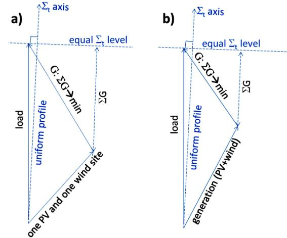
Figure 2. Load matching diagram for a) all generation is concentrated at one PV and one wind site and b) the PV and wind generation is aggregated from Western U.S. sites.
